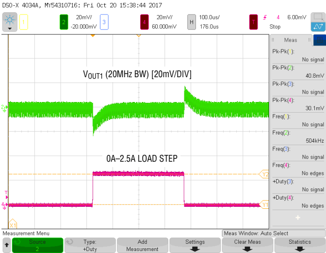
Figure 8. Output Voltage V_{OUT1} vs Load Current ( V_{OUT1} = 1.8V )
