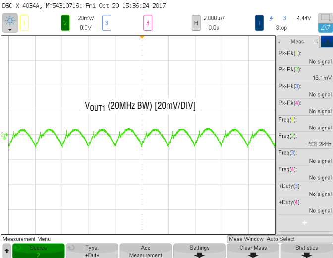
Figure 10. Output Voltage Ripple at V_{IN} = 12V , V_{OUT1} = 1.8V , I_{OUT1} = 10A
