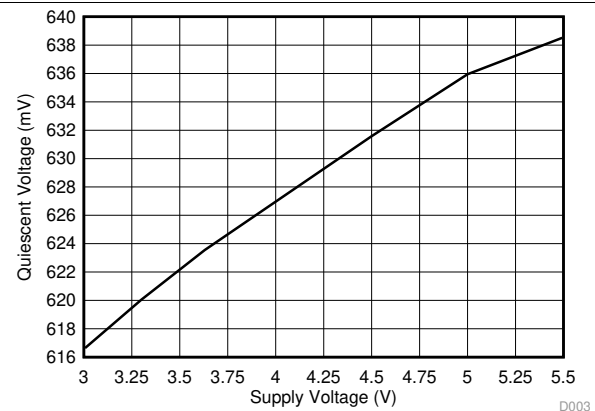
Figure 2. Quiescent Voltage vs Supply Voltage
