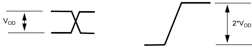
Figure 19 - Differential Voltage Parameter
