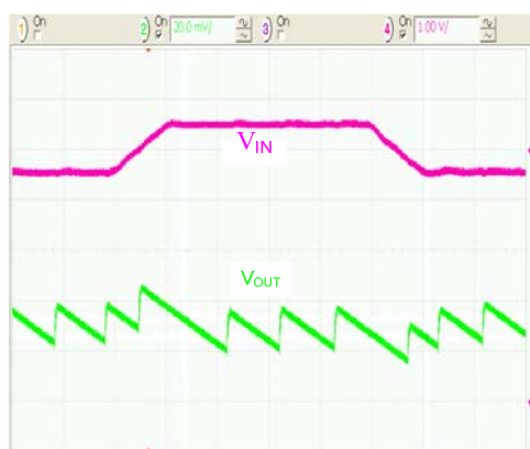
Figure 22. Line Transient Response in PFM Mode, 10\text{ }\mu\text{s/div} .
