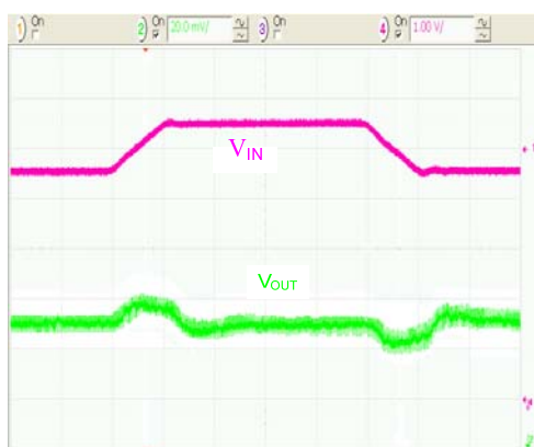
Figure 21. Line Transient Response in PWM Mode, 10\text{ }\mu\text{s/div} .
