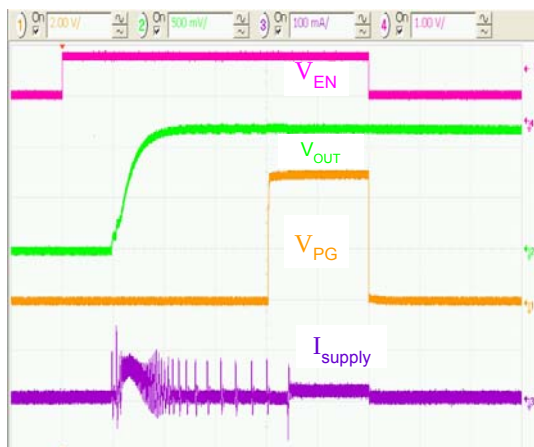
Figure 17. Soft-Start, EN Voltage Raised After V_{IN}=5\text{ V} , I_{LOAD}=0 , 100 \mu\text{s}/\text{div} .
