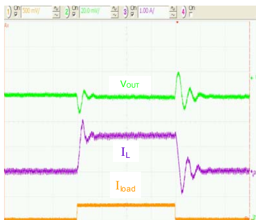
Figure 15. MODE=1, 100 mA to 1.5 A to 100 mA, 5 \mu\text{s}/\text{div} .
