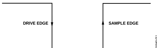
Figure 32. SPI Mode 3 SCLK Edges
