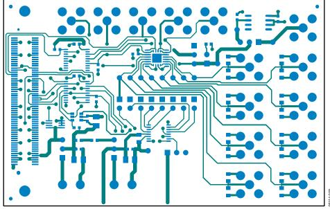
Figure 8. Component Side PCB Drawing
