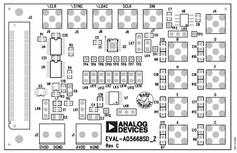
Figure 7. Component Placement Drawing
