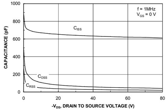
Figure 8. Capacitance Characteristics.
