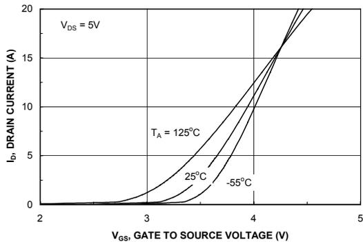
Figure 5. Transfer Characteristics.
