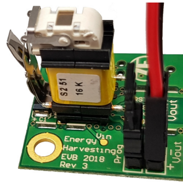
Figure 6. Power Connection and Programming Mode Jumper
