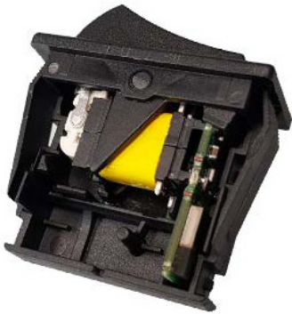
Figure 5. Rocker Switch with Bluetooth Low Energy Module
