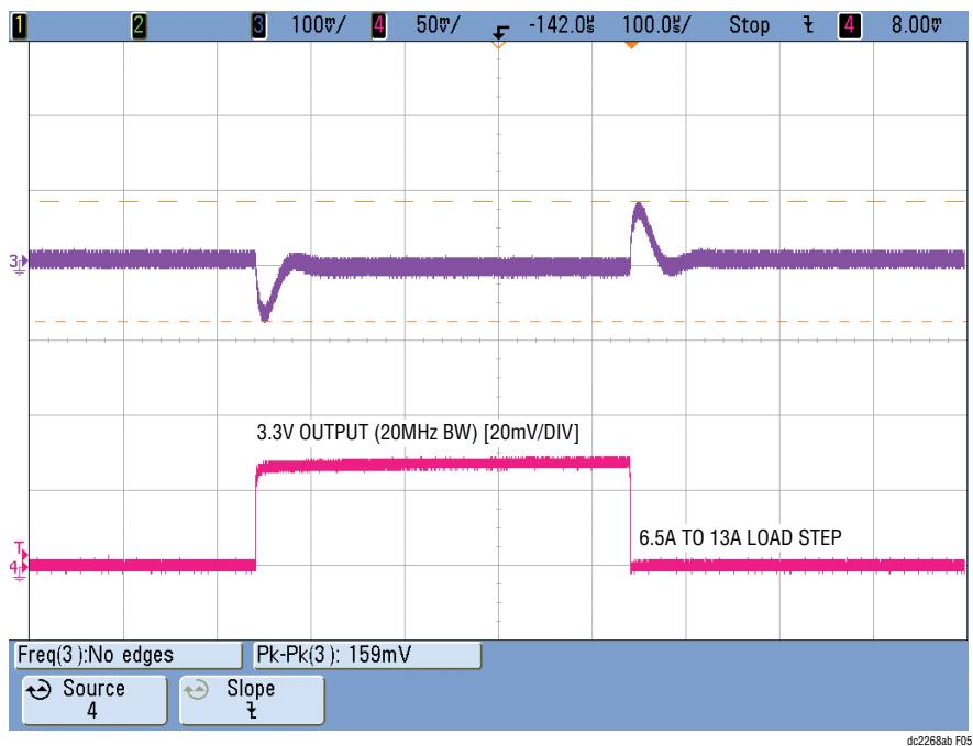
Figure 5. Measured Channel 6.5A to 13A Load Transient (V IN = 12V, V OUT1 = 3.3V)
