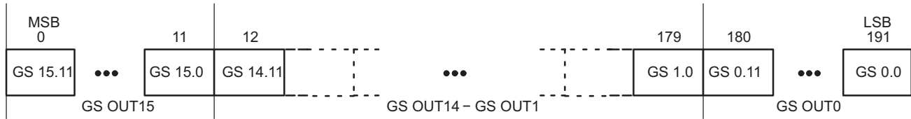
Figure 11. Grayscale Data Packet Format
