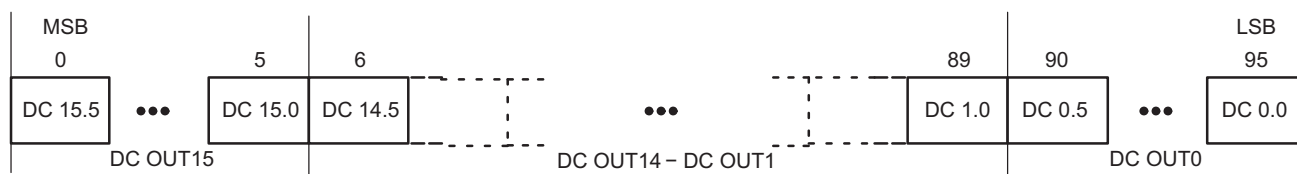
Figure 9. Dot Correction Data Packet Format
