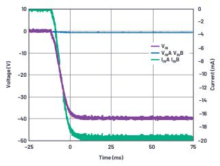
Figure 10. Reverse voltage protection measurement.
