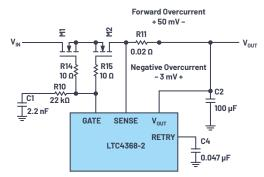
Figure 6. Application overcurrent and inrush current protection.
