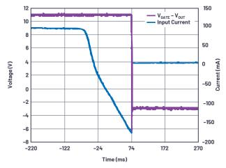
Figure 13. Assertion of reverse overcurrent protection.
