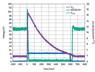
Figure 9. Complete load dump waveform.
