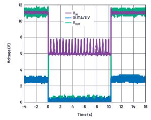
Figure 7. Complete cranking waveform.
