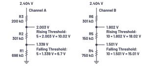
Figure 3. Resistive divider determination for voltage monitor thresholds.
