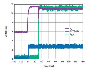
Figure 8. Expanded cranking recovery.
