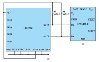
Figure 4. Range and comparator output polarity selection.
