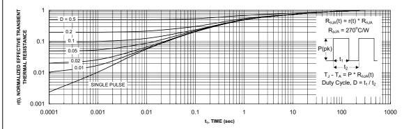
Figure 11. Transient Thermal Response Curve.
