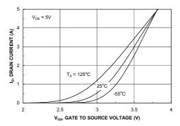
Figure 5. Transfer Characteristics.
