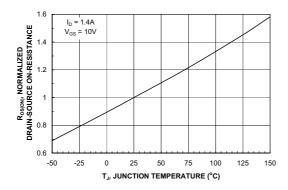
Figure 3. On-Resistance Variation with Temperature.
