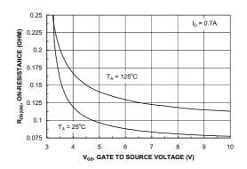
Figure 4. On-Resistance Variation with Gate-to-Source Voltage.
