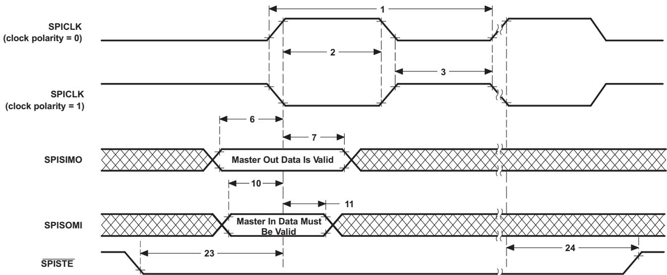
Figure 5-18. SPI Master Mode External Timing (Clock Phase = 1)
