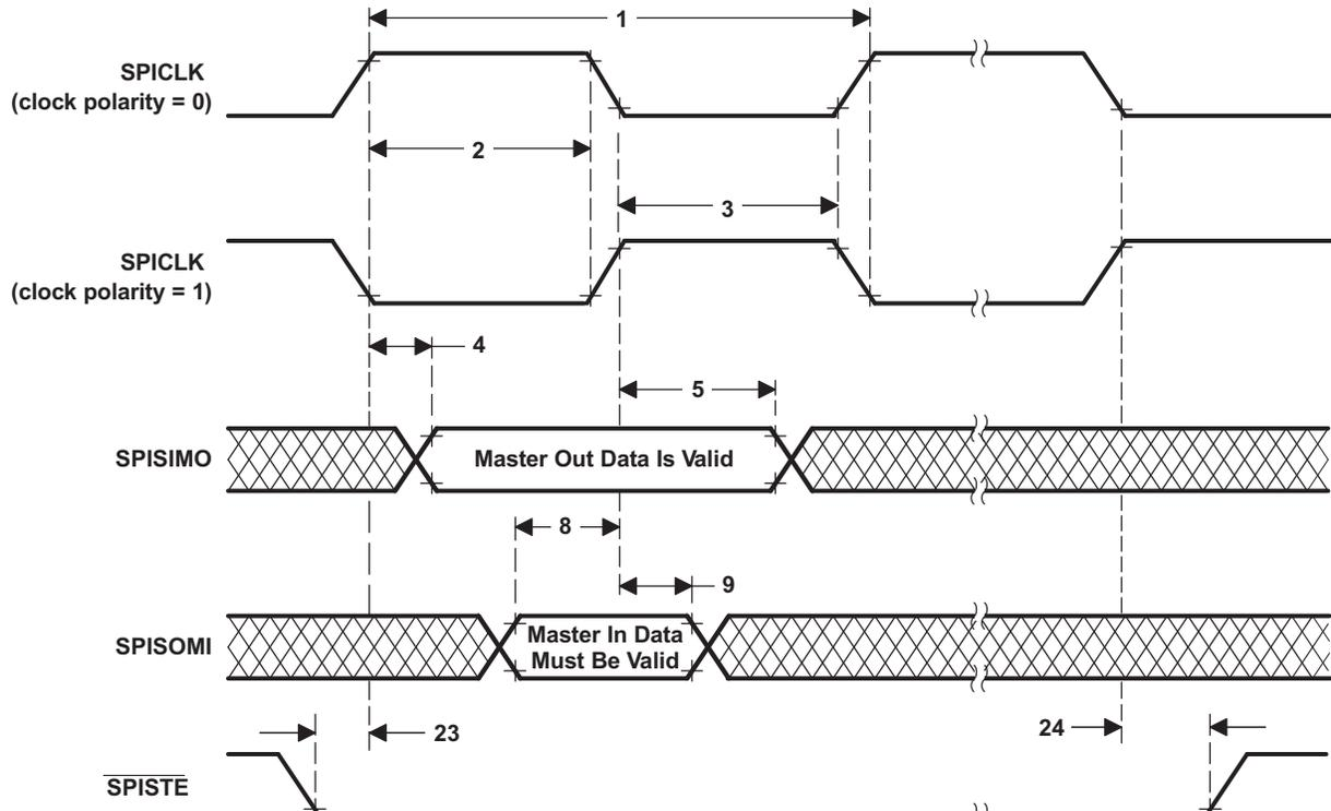
Figure 5-17. SPI Master Mode External Timing (Clock Phase = 0)
