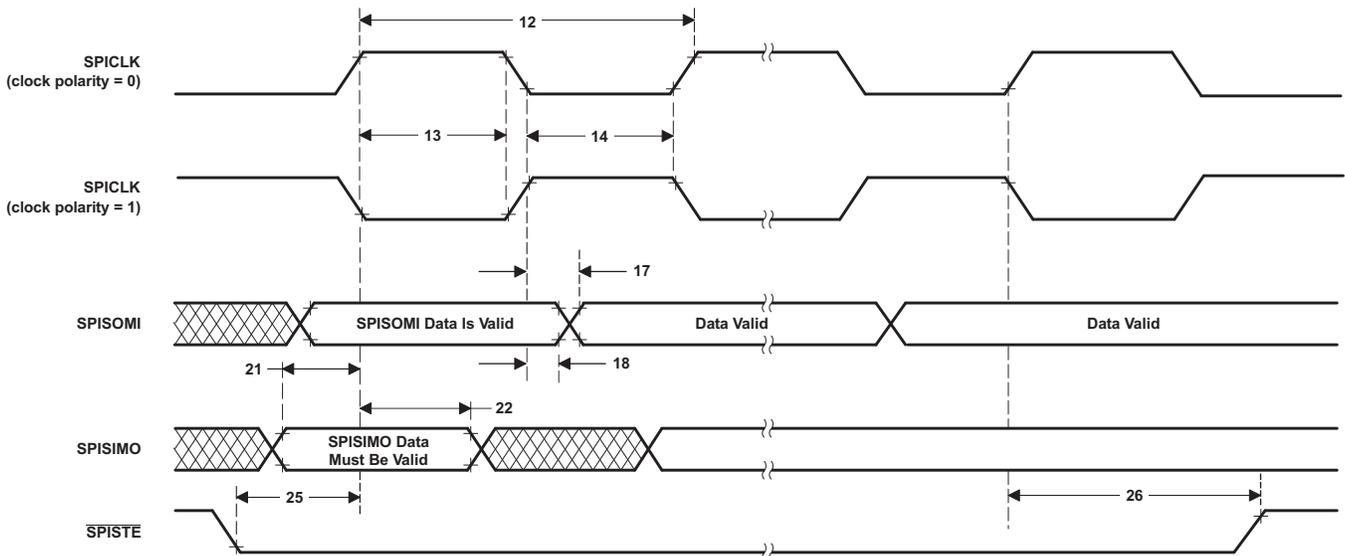
**Figure 5-20. SPI Slave Mode External Timing (Clock Phase = 1)**
