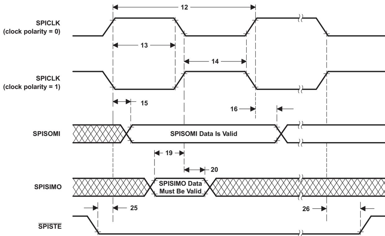
**Figure 5-19. SPI Slave Mode External Timing (Clock Phase = 0)**
