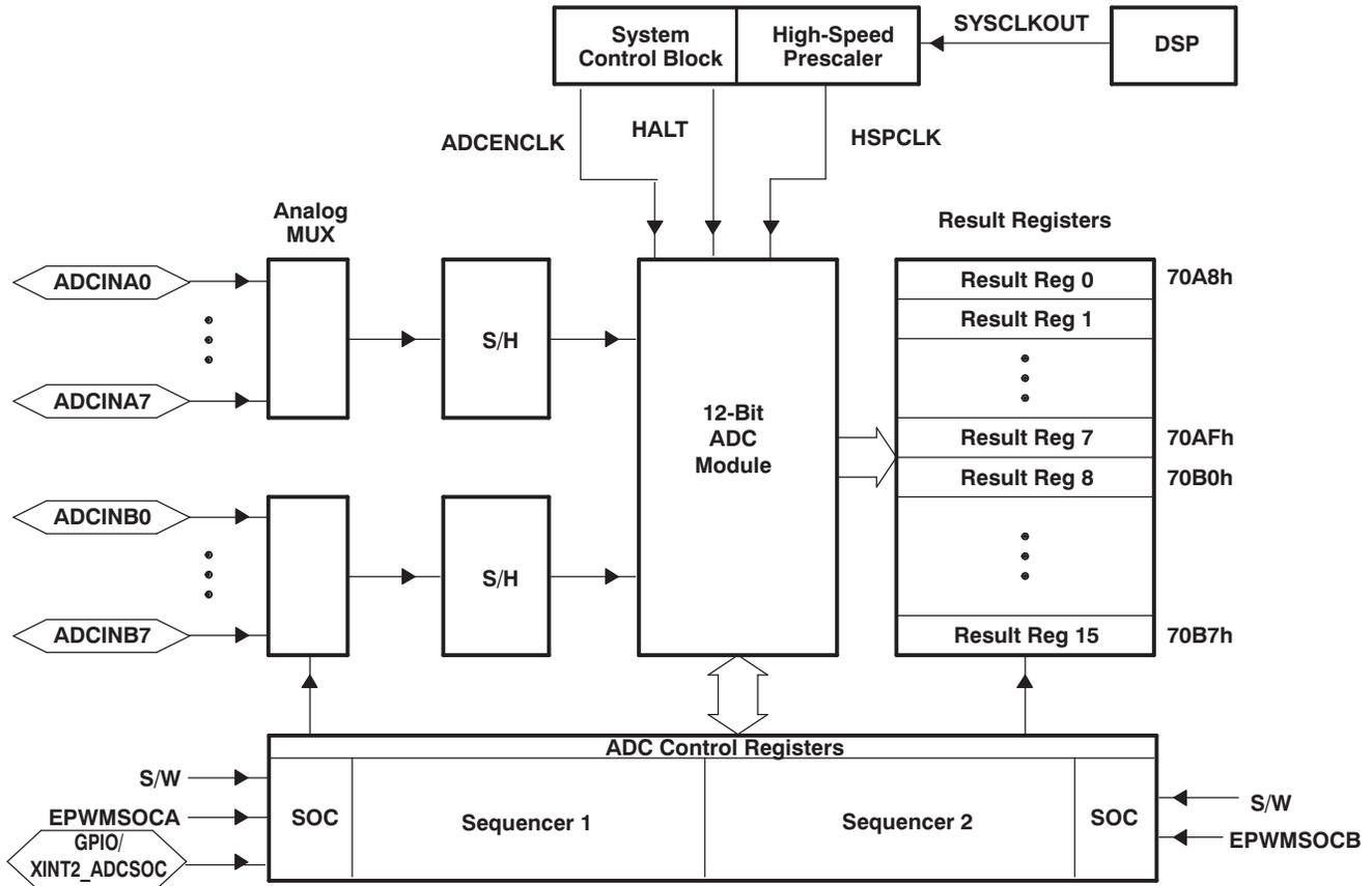
Figure 6-8. Block Diagram of the ADC Module
