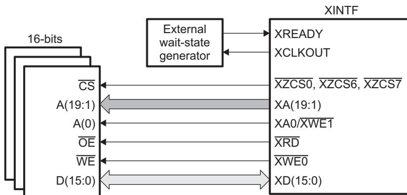
Figure 6-21. Typical 16-Bit Data Bus XINTF Connections
