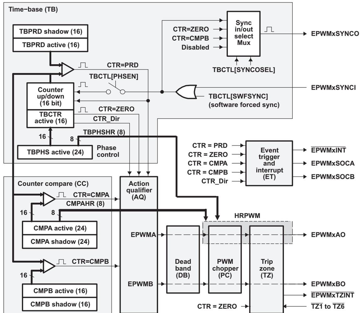
Figure 6-5. ePWM Submodules Showing Critical Internal Signal Interconnections
