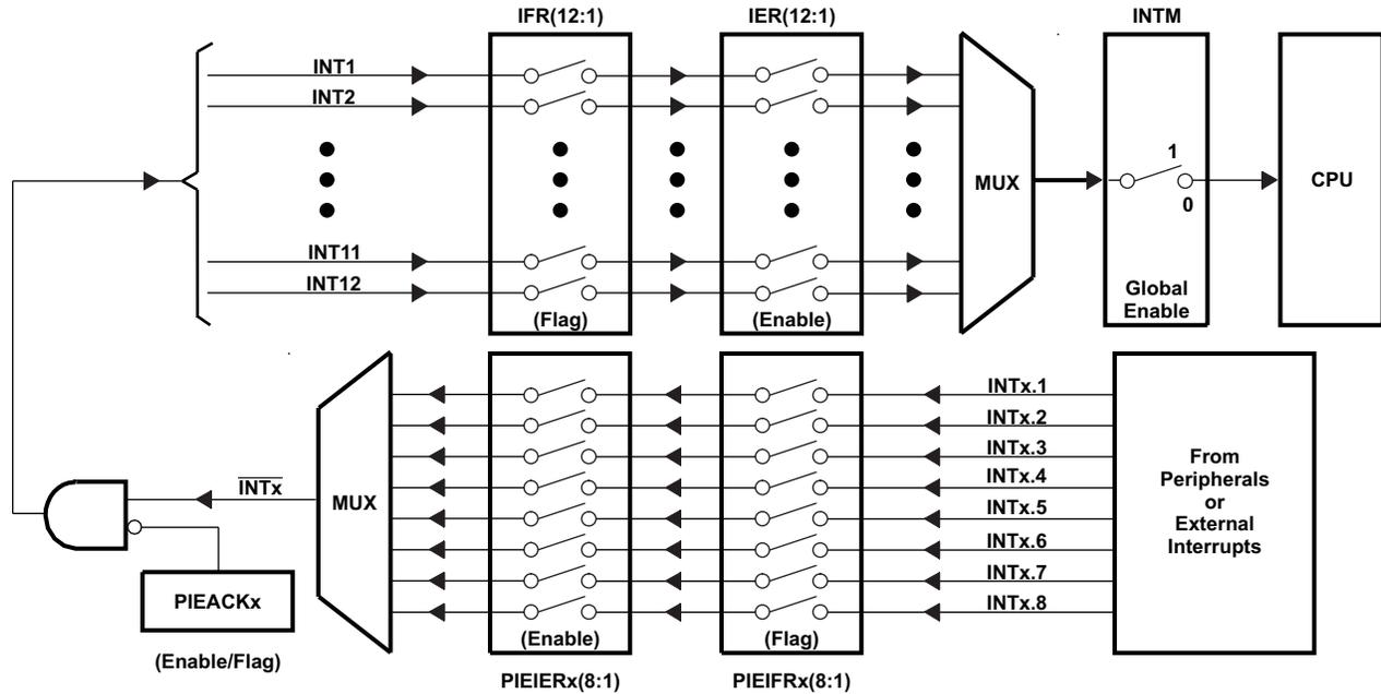
Figure 6-28. Multiplexing of Interrupts Using the PIE Block
