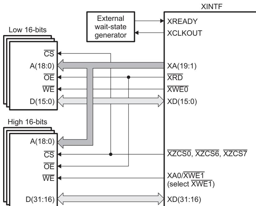
Figure 6-22. Typical 32-Bit Data Bus XINTF Connections
