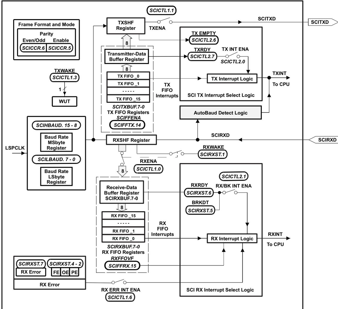
Figure 6-15. Serial Communications Interface (SCI) Module Block Diagram
