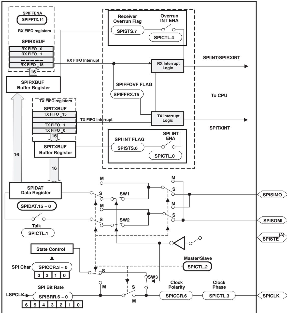
A.  $\overline{\text{SPISTE}}$  is driven low by the master for a slave device.
