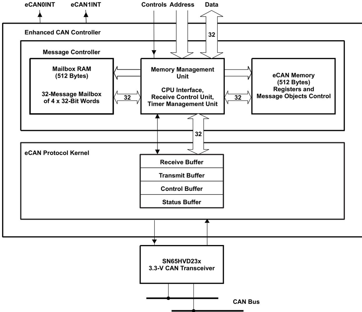
Figure 6-12. eCAN Block Diagram and Interface Circuit
