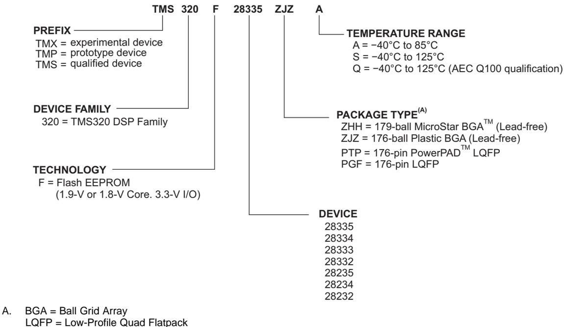
**Figure 8-1. Example of F2833x, F2823x Device Nomenclature**
