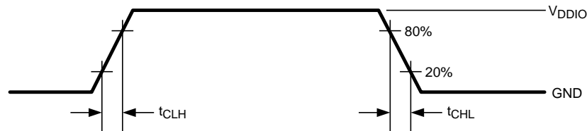
Figure 3. LVCMOS Transition Times
