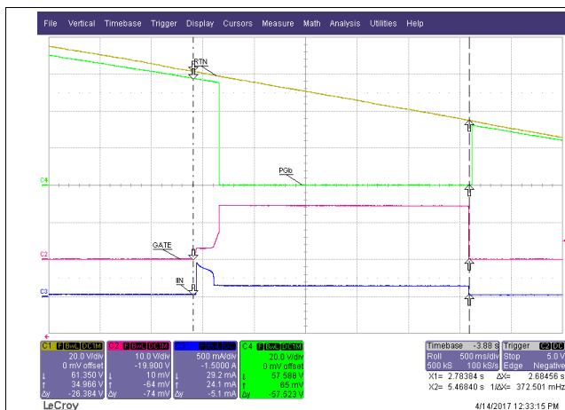
Figure 32. Plug in V_{IN,A} Backwards
