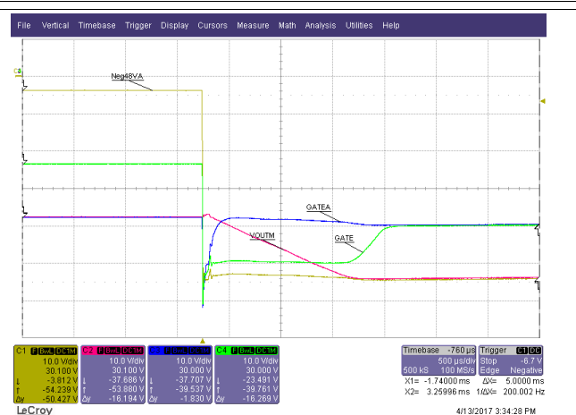
V_{IN,A} = 54\text{ V} ; V_{IN,B} = 38\text{ V} , scope GND = RTN, Iload = 5 A
