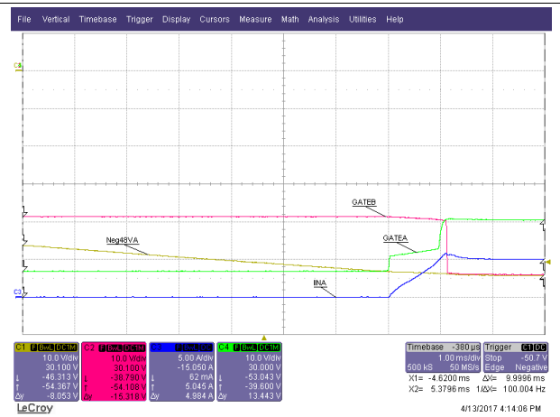
V_{INB} = 53\text{ V} (raise V_{INA} ), scope GND = RTN, Iload = 5 A
