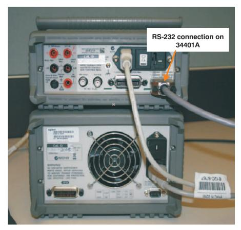
Figure 18. Connect Serial Port to DMM
