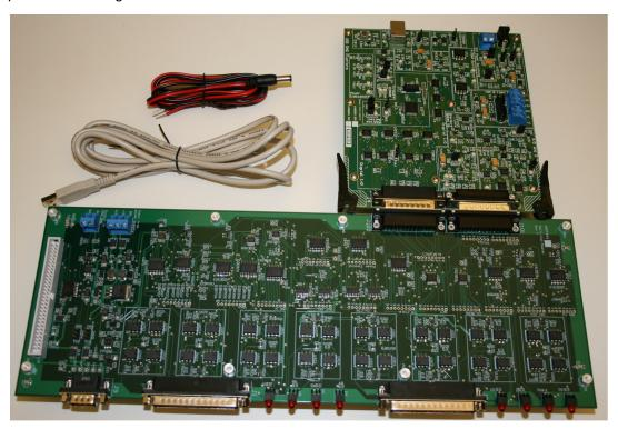
Figure 1. Hardware Included with the Multi-Cal-System EVM Kit
