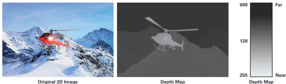
Figure 1. Time of flight (ToF): a technology to detect the distance to an object.
