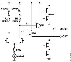
Figure 54. LVPECL Output Simplified Equivalent Circuit
