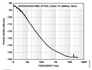
NOTES 1. THE LOOP FILTER USED TO GENERATE THIS PLOT IS SHOWN IN FIGURE 42.
