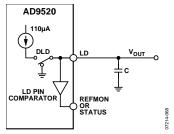
Figure 45. Current Source Digital Lock Detect
