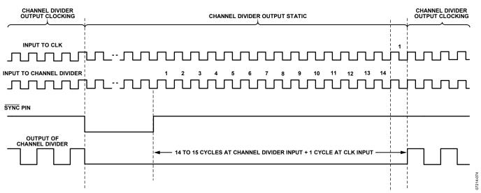
Figure 53. SYNC Timing Pipeline Delay When the VCO Divider Is Not Used—CLK Input Only
