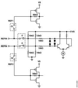
Figure 43. REFIN Equivalent Circuit for Non-XTAL Mode
