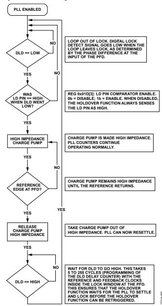
Figure 47. Flowchart of Automatic/Internal Holdover Mode
