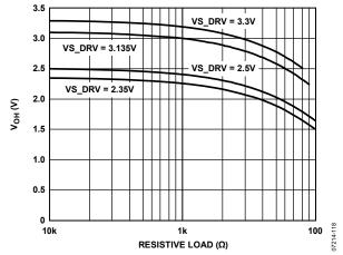
Figure 15. CMOS Output V<sub>OH</sub> (Static) vs. R<sub>LOAD</sub> (to Ground)
