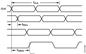
Figure 3.  $CLK/\overline{CLK}$  to Clock Output Timing, DIV = 1
