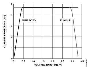
Figure 9. Charge Pump Characteristics at  $CP_V = 3.3 \text{ V}$
