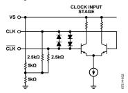
Figure 46. CLK Equivalent Input Circuit
