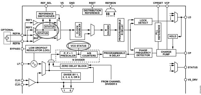
Figure 48. Reference and VCO/CLK Frequency Status Monitors
