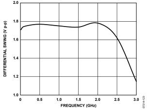
Figure 20. LVPECL Differential Voltage Swing vs. Frequency
