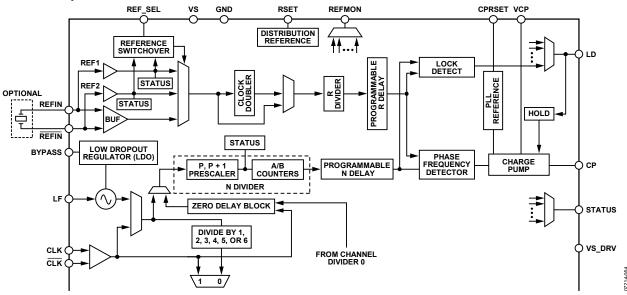
Figure 38. PLL Functional Block Diagram
