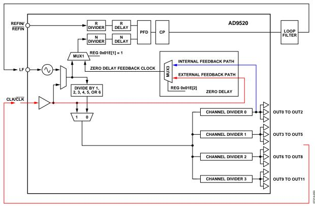
Figure 49. Zero Delay Function
