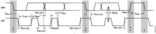
Figure 61. I<sup>2</sup>C Serial Port Timing
