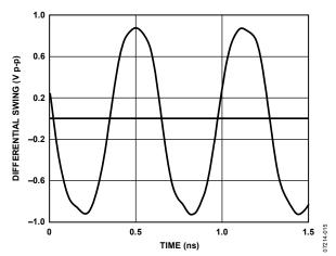
Figure 17. LVPECL Differential Voltage Swing at 1600 MHz
