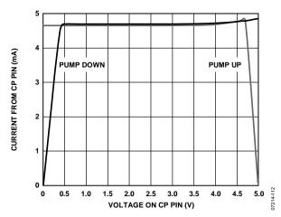
Figure 10. Charge Pump Characteristics at  $CP_V = 5.0 \text{ V}$
