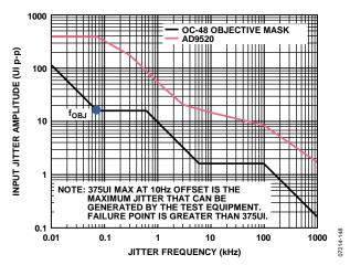
Figure 33. Telcordia GR-253 Jitter Tolerance Plot
