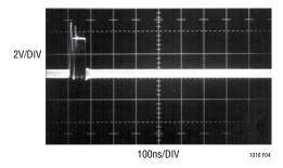
Figure 4. LT1016 Response with Poor Bypassing
