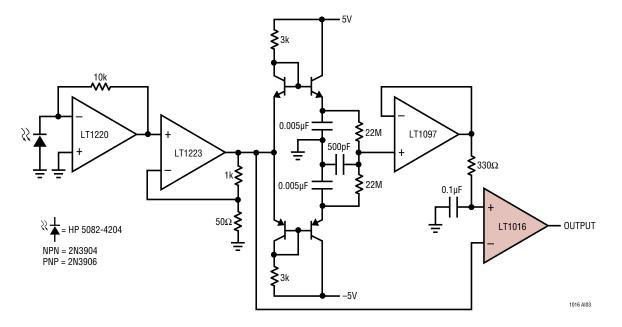
50MHz Fiber Optic Receiver with Adaptive Trigger
