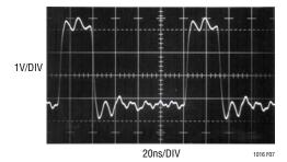
Figure 7. Typical Results Due to Poor Probe Grounding
