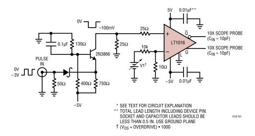
Figure 1. Response Time Test Circuit
