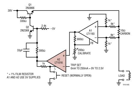
18ns Fuse with Voltage Programmable Trip Point
