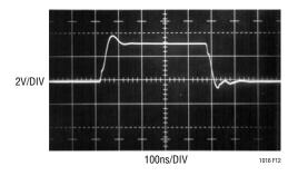
Figure 12. Excessive Load Capacitance Forces Edge Distortion
