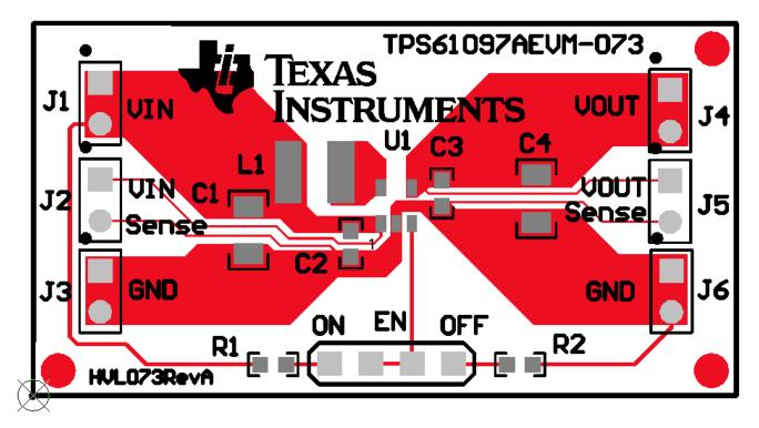
Figure 1. Top Assembly Layer
