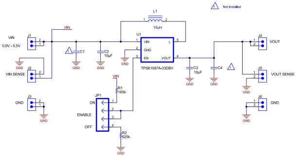
Figure 4. TPS61097AEVM-073 Schematic
