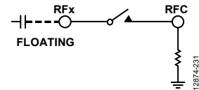
Figure 59. Series Capacitor Directly Connected to MEMS Switch
