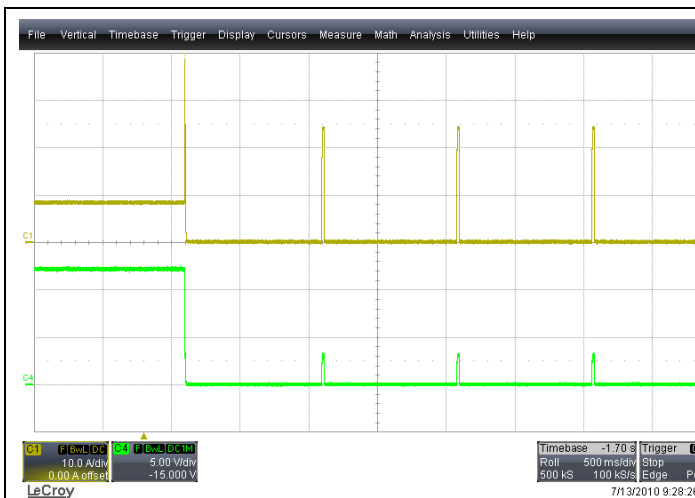
Figure 32 - Hysteretic short circuit protection, 60VDC Upper trace: Output current, 10A/div, 500ms/div Lower trace: Output Voltage, 5V/div, 500ms/div
