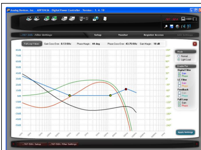
Figure 43 - Full loop gain and phase for Light Load mode
