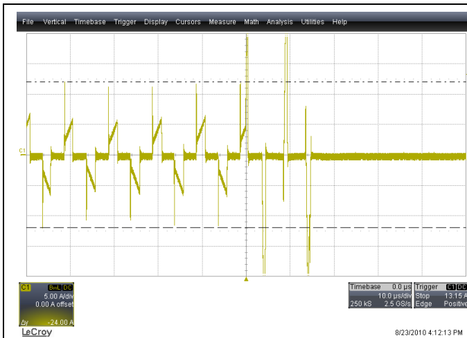
Figure 29 - Primary current during transformer short (TP16 and TP17), 60VDC. ADP1043 waits for 4 switching cycles before disabling PSU. 5A/div, 5us/div
