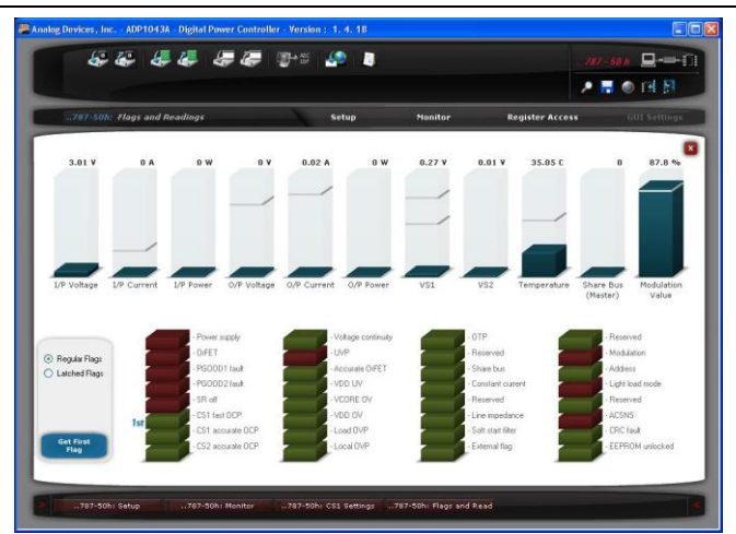
Figure 30 - Corresponding 'Flags and Readings' window. CS1 Fast OCP was the first flag that tripped
