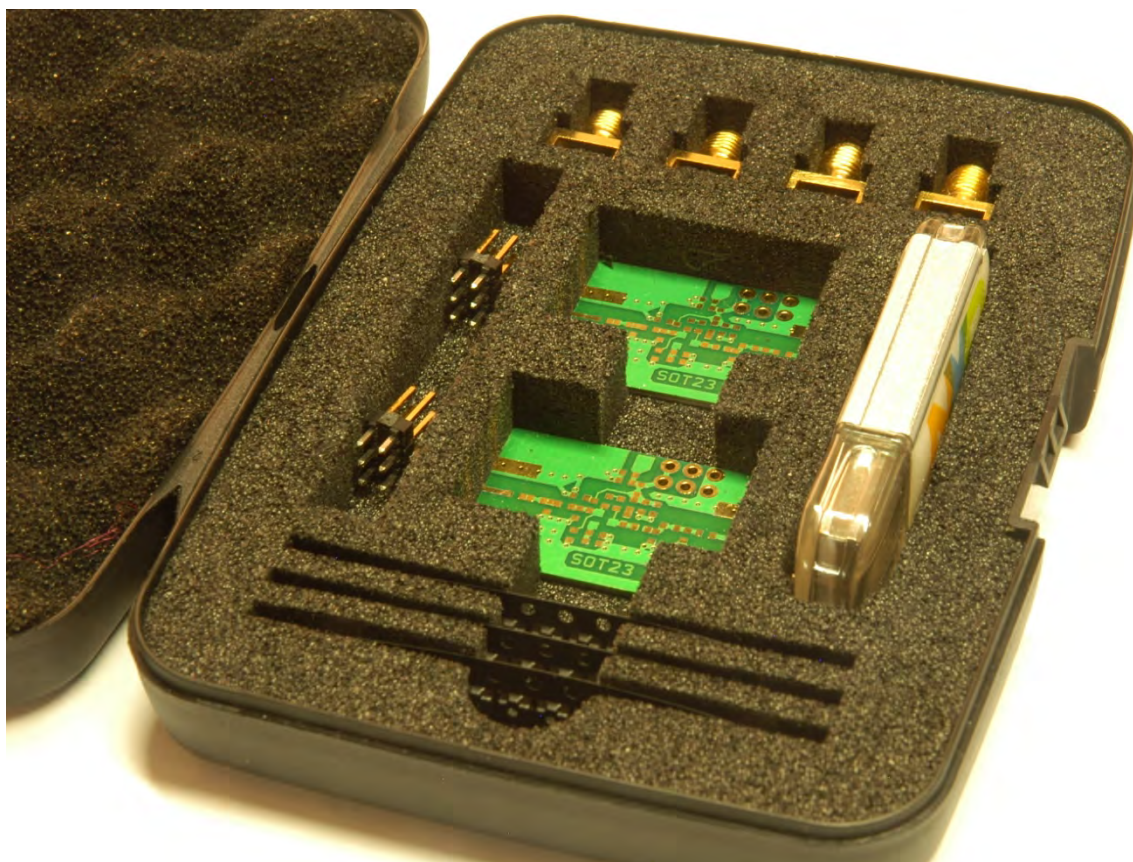
Fig 1. BFU5xx series starter kit
