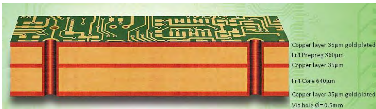
Fig 5. Applied PCB layout stack
