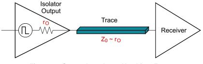
Figure 11. Source Impedance Matching:  $Z_0 \sim r_o$
