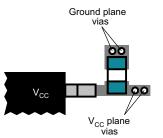
Figure 20. Connect Bypass Capacitor Directly to V<sub>cc</sub> Terminal
