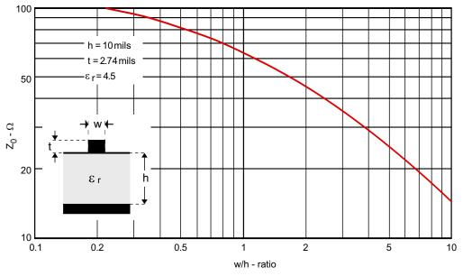
Figure 13. Characteristic Impedance as a Function of the w/h Ratio
