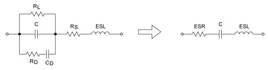
Figure 23. Capacitor Losses Modeled by a Series Resonance Circuit
