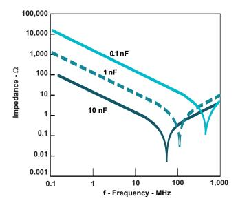
Figure 24. Capacitor Impedance Versus Frequency
