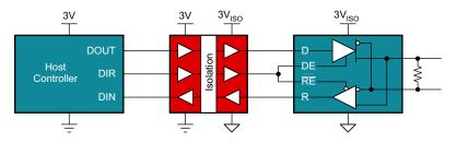
Figure 7. Isolated RS-485 Interface
