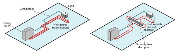
Figure 16. Return Current Paths in Solid Versus Slotted Ground Planes
