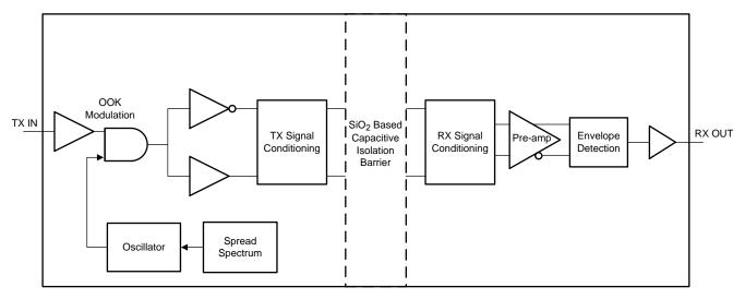
Figure 2. Conceptual Block Diagram of On-Off Keying (OOK) Architecture
