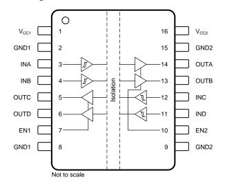
Figure 4. Example Isolator in a 16-Pin Package
