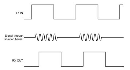
Figure 3. Representative Signal in OOK Architecture
