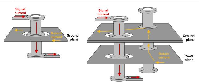
Figure 21. Return Current Paths for a Single and a Multiple Layer Change
