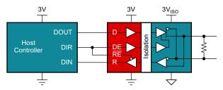
Figure 8. Integrated Isolated RS-485 Interface
