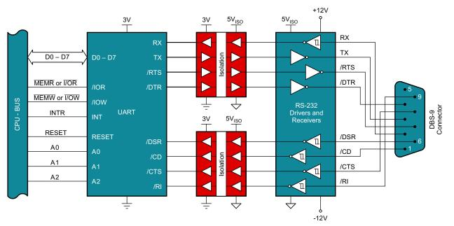
Figure 6. Isolated RS-232 Interface
