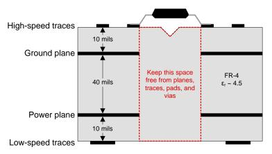
Figure 9. Recommended Layer Stack
