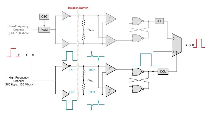
Figure 1. Conceptual Block Diagram of Edge-Based Architecture
