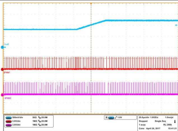
V_{VIN} = 12\text{ V} I_{VOUT\_B} = 30\text{ A} V_{OUT\_B} VID step from 0.8 V to 1.2 V
