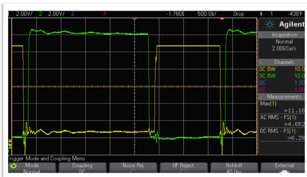
Figure 10: 3.3V/25W Flyback Primary and secondary FETs Gate
