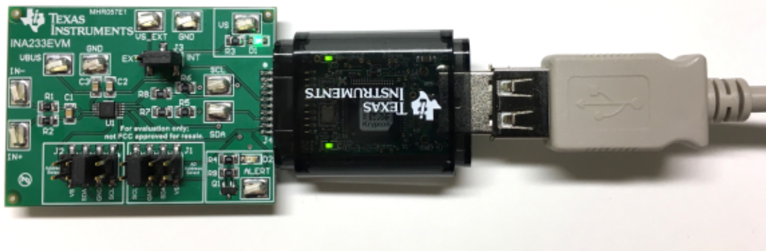
Figure 10. INA233 Power-Up using SM_USB DIG and INA233EVM GUI Software
