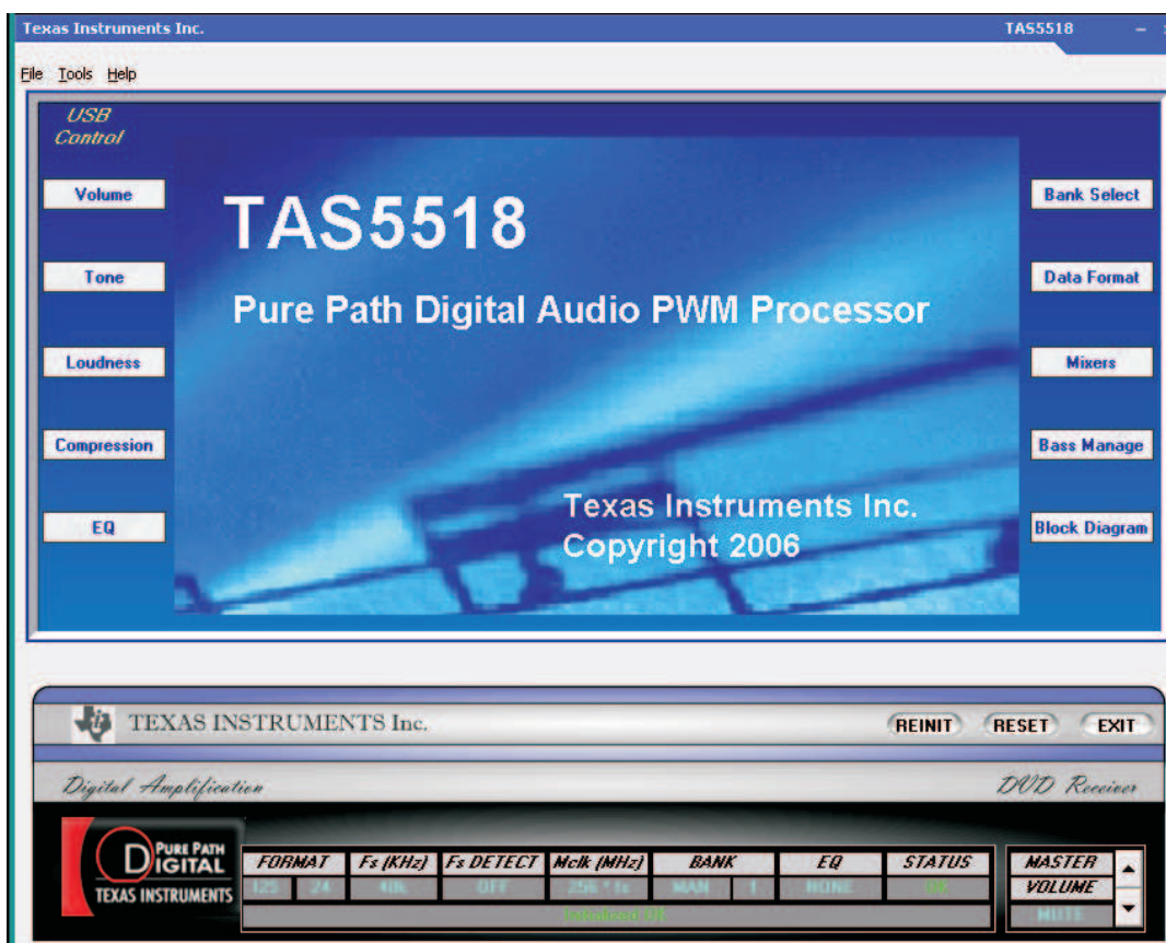
Figure 3. TAS5518 GUI Window
