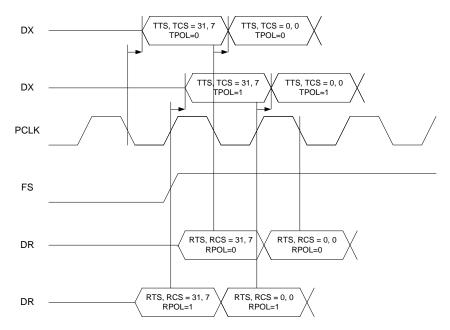
Figure 1: 73M1866B/73M1966B PCM Frame Bit Numbering
