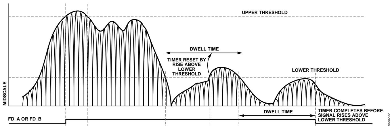
Figure 89. Threshold Settings for FD\_A and FD\_B Signals
