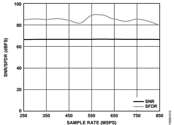
Figure 37. SNR/SFDR vs. Sample Rate,  $f_{IN} = 172.3$  MHz
