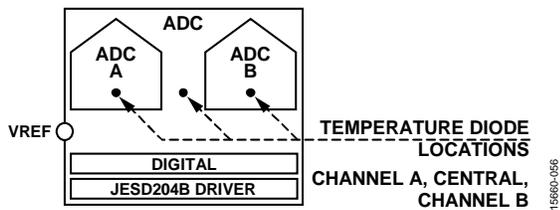
Figure 85. Temperature Diode Locations in the Die
