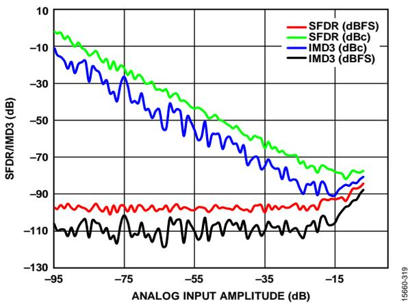
Figure 20. SFDR/IMD3 vs. Analog Input Amplitude,  $f_{IN} = 172.3$  MHz
