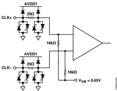
Figure 58. Clock Inputs
