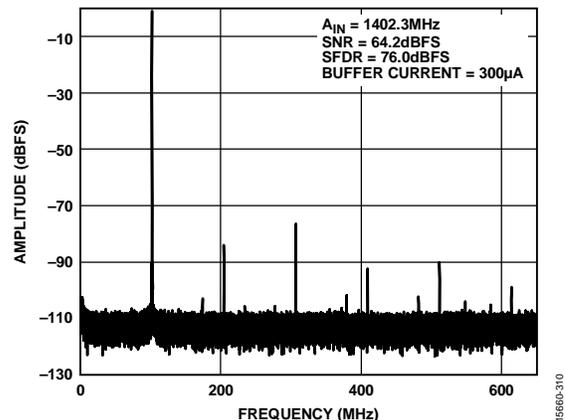
Figure 11. Single-Tone FFT with  $f_{IN} = 1402.3$  MHz
