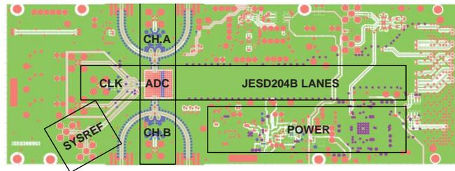
Figure 145. Recommended PCB Layout for the AD9695
