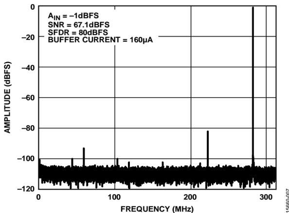
Figure 34. Single-Tone FFT with  $f_{IN} = 340$  MHz
