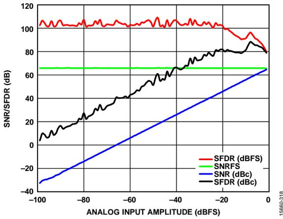
Figure 19. SNR/SFDR vs. Analog Input Amplitude,  $f_{IN} = 172.3$  MHz
