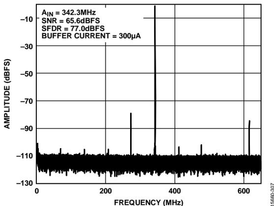
Figure 8. Single-Tone FFT with  $f_{IN} = 342.3$  MHz
