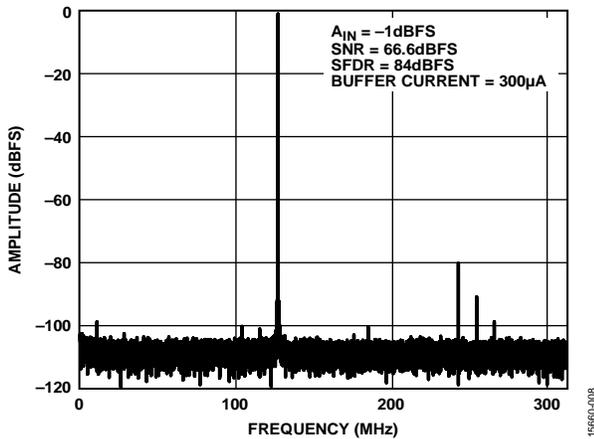
Figure 35. Single-Tone FFT with  $f_{IN} = 750$  MHz
