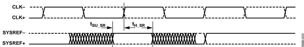
Figure 3. SYSREF± Setup and Hold Timing Diagram
