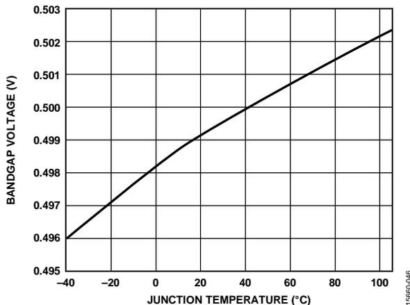
Figure 75. Typical V<sub>REF</sub> Drift
