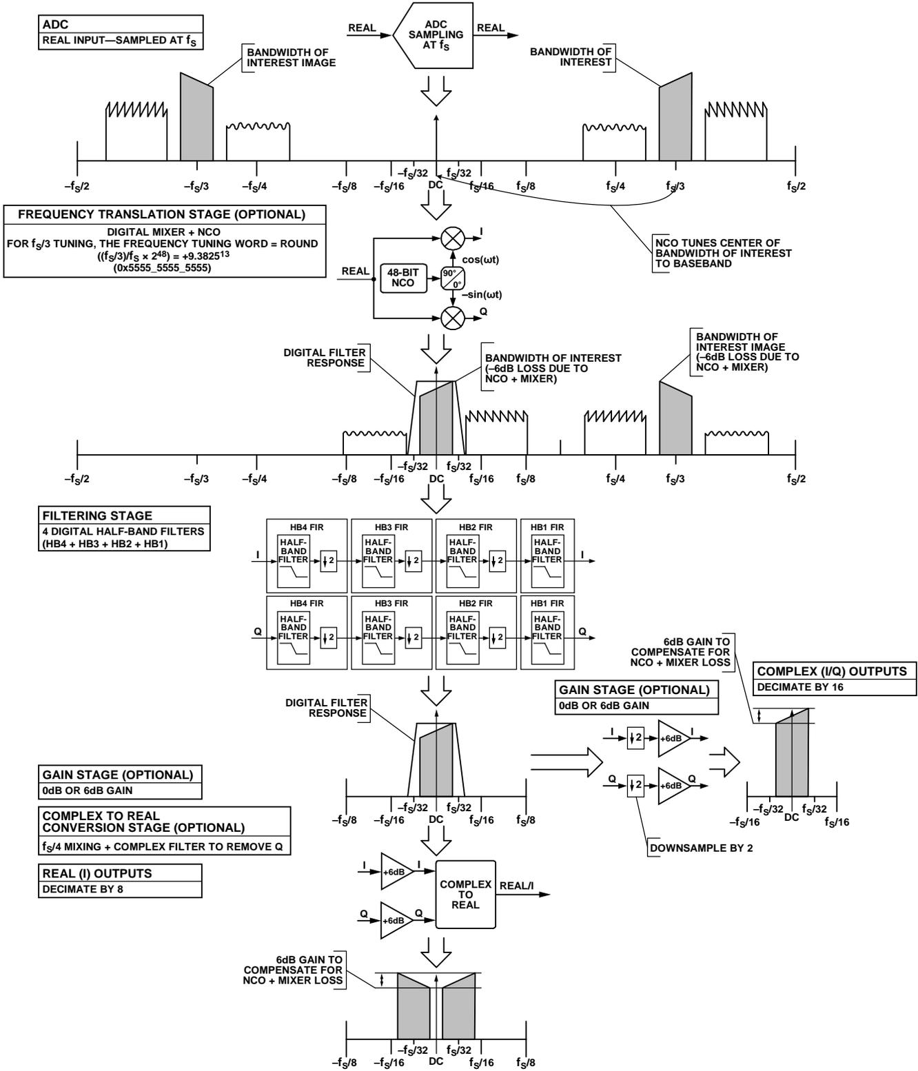
Figure 98. DDC Theory of Operation Example (Real Input)
