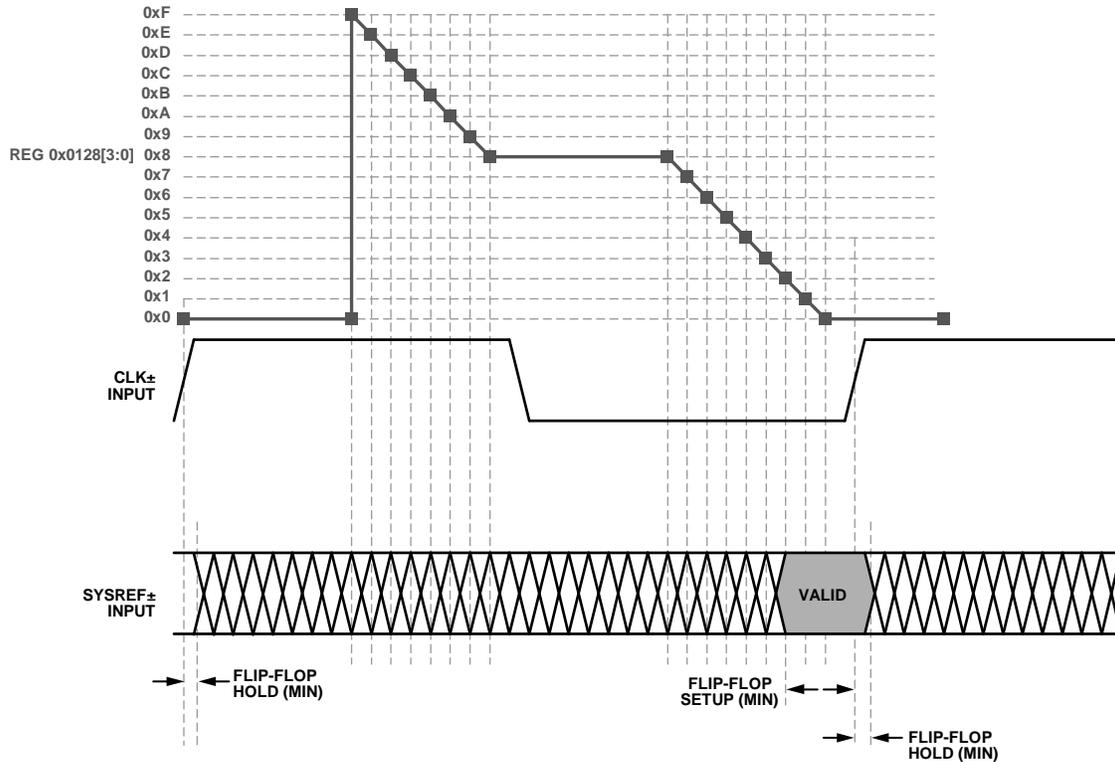
Figure 140. SYSREF± Setup Detector
