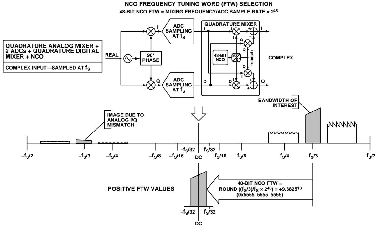
Figure 100. DDC NCO Frequency Tuning Word Selection—Complex Inputs
