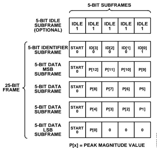
Figure 117. SPORT over JESD204B Signal Monitor Frame Data
