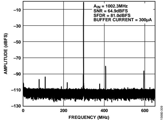
Figure 10. Single-Tone FFT with  $f_{IN} = 1002.3$  MHz
