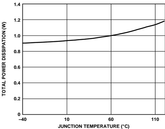
Figure 47. Total Power Dissipation vs. Junction Temperature
