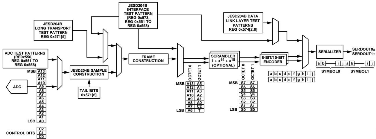
Figure 142. ADC Output Datapath Showing Data Framing
