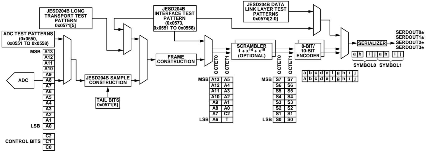
Figure 120. ADC Output Datapath Showing Data Framing
