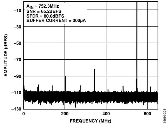
Figure 9. Single-Tone FFT with  $f_{IN} = 752.3$  MHz
