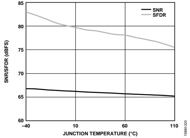
Figure 21. SNR/SFDR vs. Junction Temperature,  $f_{IN} = 172.3$  MHz
