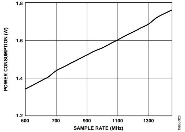
Figure 27. Total Power Dissipation vs. Sample Rate ( $f_s$ )
