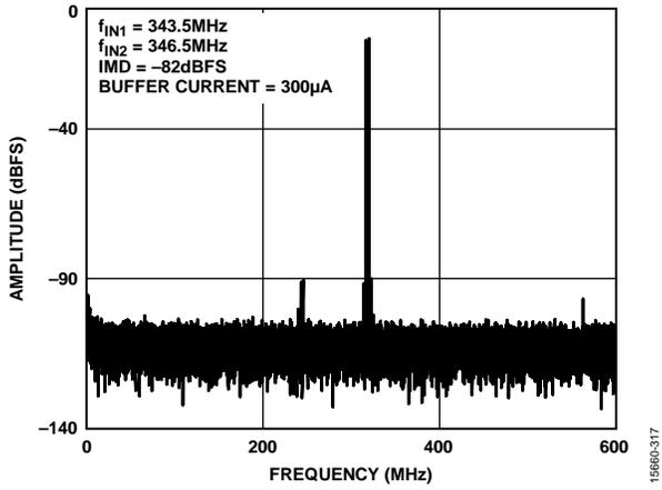
Figure 18. Two-Tone FFT;  $f_{IN1} = 343.5$  MHz,  $f_{IN2} = 346.5$  MHz
