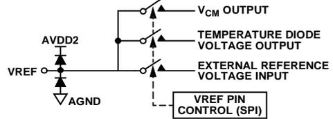
Figure 66. VREF Input/Output
