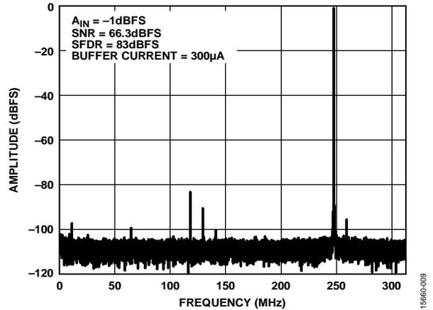
Figure 36. Single-Tone FFT with  $f_{IN} = 1000$  MHz
