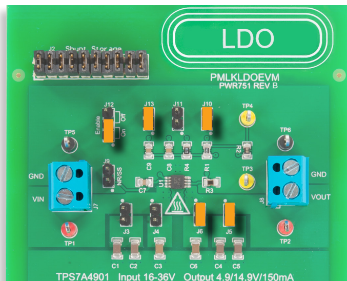
Figure 7. TPS7A4901 LDO board: jumpers set-up for Test#2
