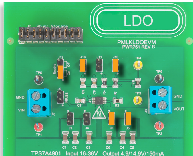
Figure 6. TPS7A4901 LDO board: jumpers set-up for Test#1
