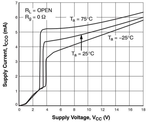
Figure 48.  $I_{CCO} - V_{CC}$
