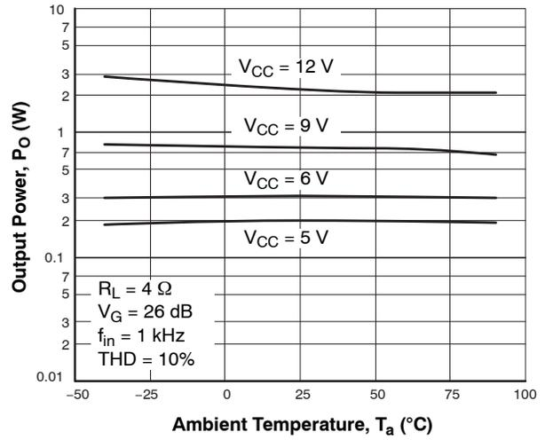
Figure 42. P<sub>O</sub> - T<sub>a</sub>
