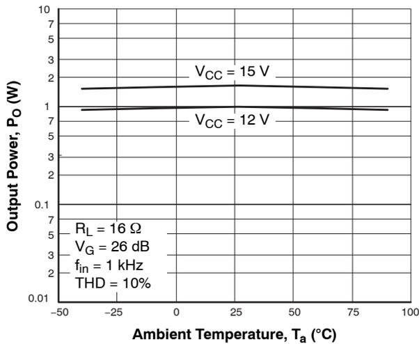
Figure 43. P<sub>O</sub> - T<sub>a</sub>
