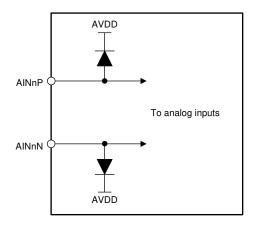
Figure 20. Input ESD Protection Circuitry
