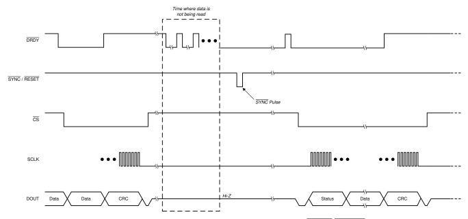
Figure 38. Collecting Data After a Hiatus Using the SYNC/RESET Pin
