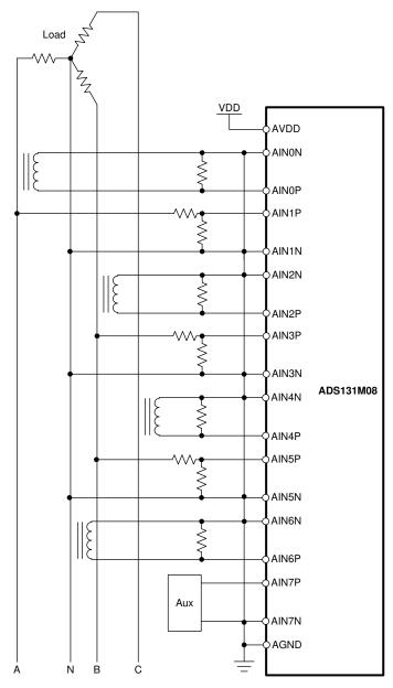
Figure 99. Three-Phase Metrology Design Front-End
