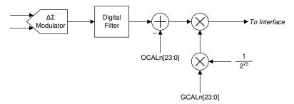
Figure 32. Calibration Block Diagram
