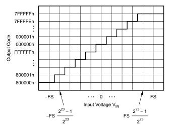
Figure 37. Code Transition Diagram
