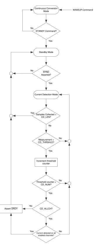
Figure 35. Current-Detect Mode Flow Chart
