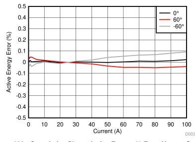
Figure 102. Cumulative Phase Active Energy % Error Versus Current
