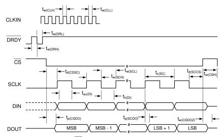
NOTE: SPI settings are CPOL = 0 and CPHA = 1.  $\overline{\text{CS}}$  transitions must take place when SCLK is low.
