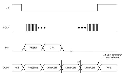
Figure 40. RESET Command Frame
