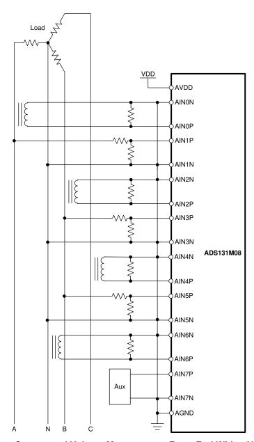
Figure 97. Three-Phase Current and Voltage Measurement Front-End With a Neutral Current Monitor
