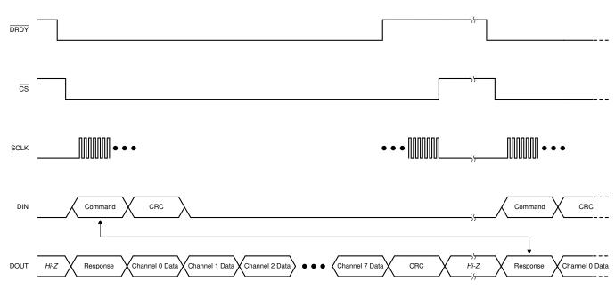
Figure 36. Typical Communication Frame
