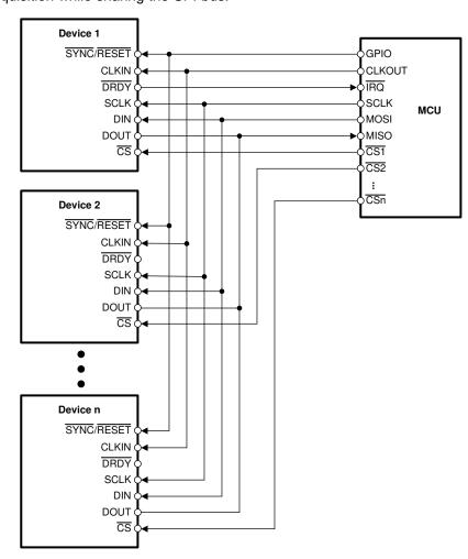
Figure 98. Multiple Device Configuration
