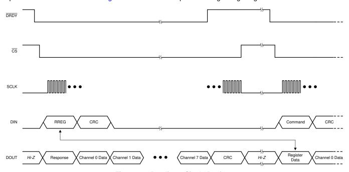
Figure 41. Reading a Single Register
