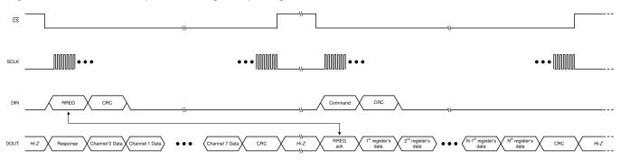
Figure 42. Reading Multiple Registers
