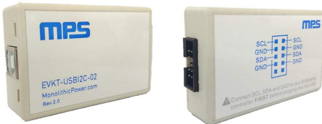
**Figure 3: EVKT-USBI2C-02 Communication Interface Device**
