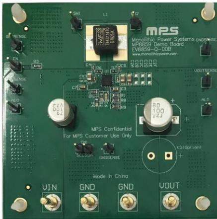
**Figure 2: EV8859-Q-00B Evaluation Board**
