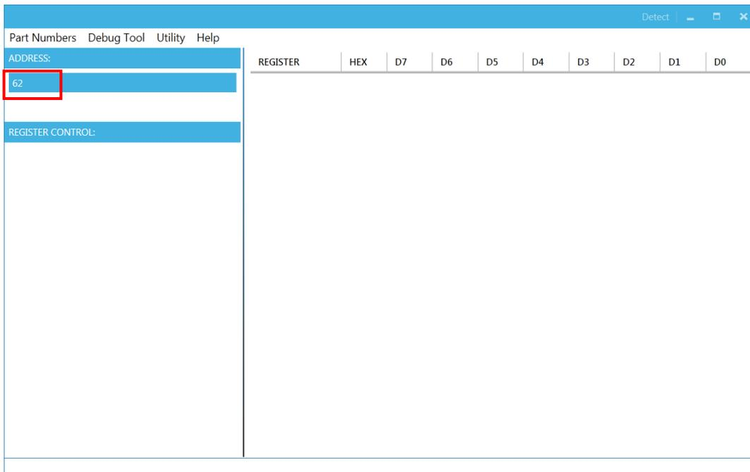
**Figure 7: Appearance of Address Shows Successful Connection**
