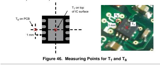
**NOTE** Both  $T_T$  and  $T_B$  can be measured on actual application boards using an infrared thermometer.
