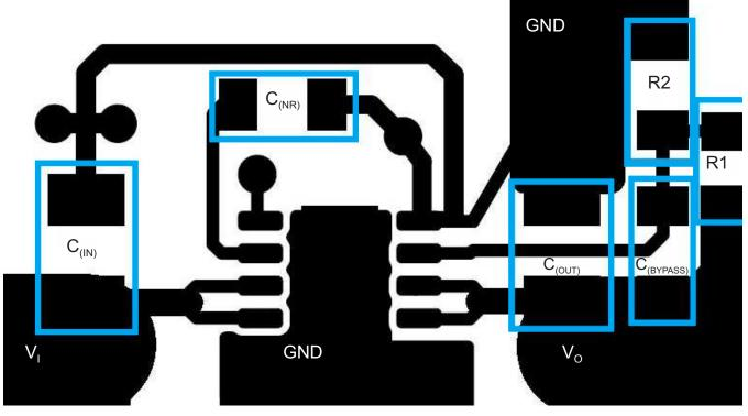
Figure 44. TPS7A8101-Q1 Layout Example
