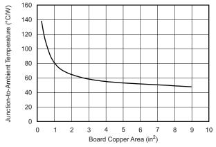
Note: The  $R_{\theta,JA}$  value at board size of 9 in<sup>2</sup> (that is, 3 in × 3 in) is a JEDEC standard.
