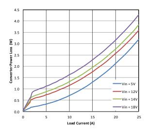
Figure 5. Power Loss of 1-V Output vs Load
