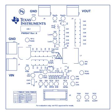
Figure 14. PWR-847EVM Top Layer Assembly Drawing (Top View)
