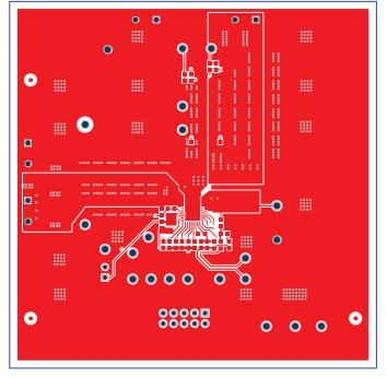
Figure 16. PWR-847EVM Top Layer (Top View)
