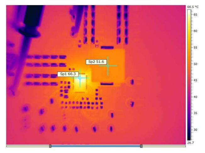
Figure 13. Thermal Image at 1-V Output at 12 V<sub>IN</sub>, 25-A Output, at 25°C Ambient
