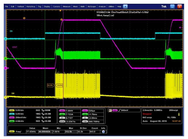
Figure 12. Output Voltage Start-up and Shutdown, 1-V Output at 1 2V<sub>IN</sub>, 0.5-A Output
