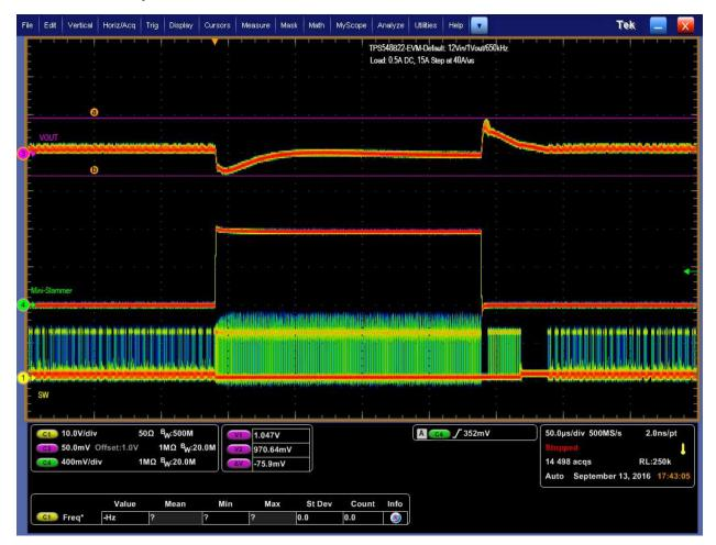
Figure 7. Transient Response of 1-V Output at 12  $V_{\mbox{\tiny IN}},$  Transient is 0.5 A to 15.5 A, the Step is 15 A at 40 A/µs
