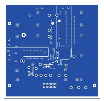
Figure 21. PWR-847EVM Bottom Layer (Top View)
