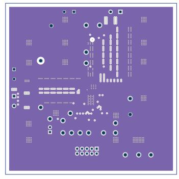
Figure 20. PWR-847EVM Inner Layer 4 (Top View)
