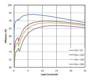
Figure 4. Efficiency of 1-V Output vs Load
