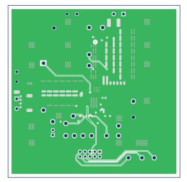
Figure 19. PWR-847EVM Inner Layer 3 (Top View)
