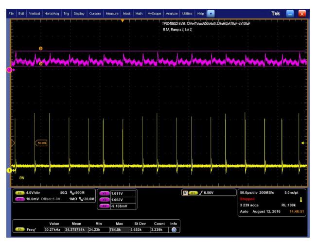
Figure 9. Output Ripple and SW Node of 1-V Output at 12 V<sub>IN</sub>, 0-A Output
