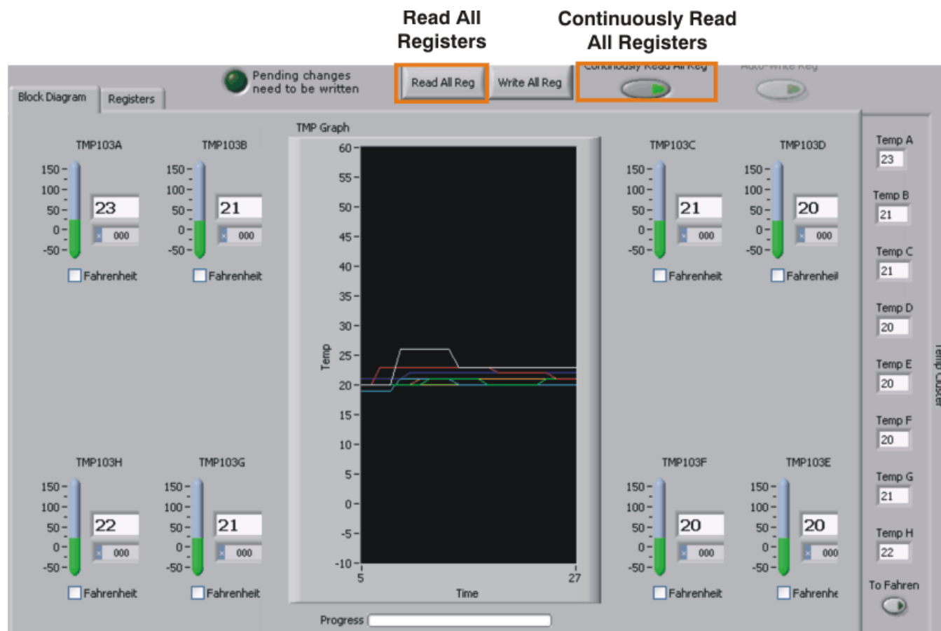
Figure 16. TMP103EVM Software: Reading from Registers
