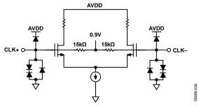
Figure 41. Equivalent Clock Input Circuit
