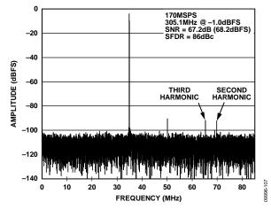
Figure 7. AD9634-170 Single-Tone FFT with  $f_{IN}$  = 305.1 MHz
