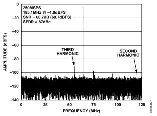
Figure 29. AD9634-250 Single-Tone FFT with  $f_{IN} = 185.1$  MHz
