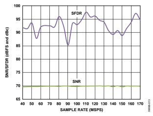
Figure 14. AD9634-170 Single-Tone SNR/SFDR vs. Sample Rate ( $f_s$ ) with  $f_{IN} = 90$  MHz
