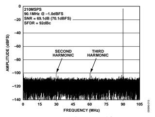
Figure 16. AD9634-210 Single-Tone FFT with  $f_{IN} = 90.1$  MHz
