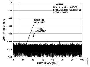
Figure 18. AD9634-210 Single-Tone FFT with  $f_{IN}$  = 220.1 MHz
