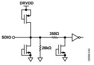
Figure 43. Equivalent SDIO Circuit
