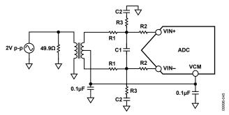
Figure 48. Differential Transformer-Coupled Configuration
