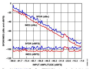
Figure 34. AD9634-250 Two-Tone SFDR/IMD3 vs. Input Amplitude (A<sub>IN</sub>) with  $f_{\rm IN1}=89.12$  MHz,  $f_{\rm IN2}=92.12$  MHz,  $f_{\rm S}=250$  MSPS
