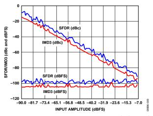
Figure 10. AD9634-170 Two-Tone SFDR/IMD3 vs. Input Amplitude (A<sub>IN</sub>) with  $f_{\rm IN1}=89.12$  MHz,  $f_{\rm IN2}=92.12$  MHz,  $f_{\rm S}=170$  MSPS
