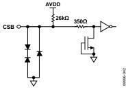
Figure 45. Equivalent CSB Input Circuit
