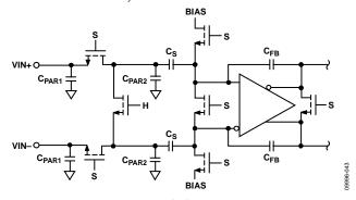
Figure 46. Switched-Capacitor Input
