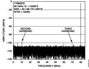
Figure 4. AD9634-170 Single-Tone FFT with  $f_{IN} = 90.1$  MHz
