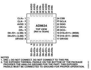
Figure 3. Pin Configuration
