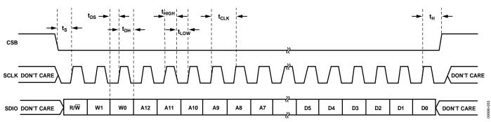
Figure 58. Serial Port Interface Timing Diagram
