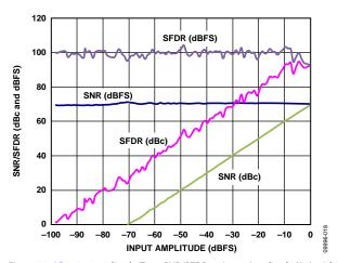
Figure 20. AD9634-210 Single-Tone SNR/SFDR vs. Input Amplitude (A<sub>IN</sub>) with  $f_{\rm IN}=90.1$  MHz,  $f_{\rm S}=210$  MSPS
