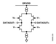
Figure 42. Equivalent LVDS Output Circuit
