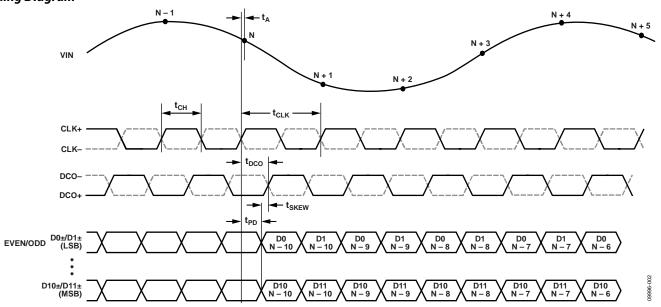
Figure 2. Even/Odd LVDS Mode Data Output Timing
