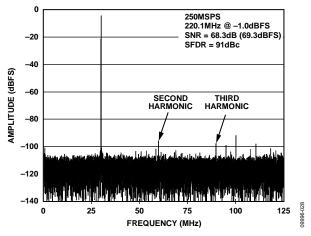
Figure 30. AD9634-250 Single-Tone FFT with  $f_{IN}$  = 220.1 MHz
