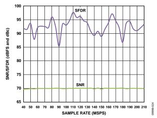
Figure 26. AD9634-210 Single-Tone SNR/SFDR vs. Sample Rate ( $f_s$ ) with  $f_{\rm IN} = 90~{\rm MHz}$
