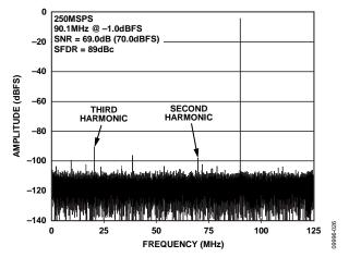
Figure 28. AD9634-250 Single-Tone FFT with  $f_{IN} = 90.1$  MHz
