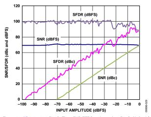
Figure 32. AD9634-250 Single-Tone SNR/SFDR vs. Input Amplitude (A<sub>IN</sub>) with  $f_{\rm IN}=90.1$  MHz,  $f_{\rm S}=250$  MSPS
