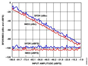
Figure 23. AD9634-210 Two-Tone SFDR/IMD3 vs. Input Amplitude (A<sub>IN</sub>) with  $f_{\rm IN1}=184.12$  MHz,  $f_{\rm IN2}=187.12$  MHz,  $f_{\rm S}=210$  MSPS
