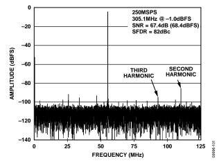
Figure 31. AD9634-250 Single-Tone FFT with  $fl_N = 305.1 \text{ MHz}$
