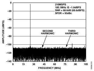
Figure 17. AD9634-210 Single-Tone FFT with  $f_{IN} = 185.1$  MHz
