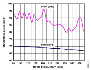
Figure 21. AD9634-210 Single-Tone SNR/SFDR vs. Input Frequency ( $f_{\mathbb{N}}$ ),  $f_{S} = 210$  MSPS
