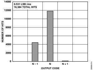
Figure 15. AD9634-170 Grounded Input Histogram,  $f_S = 170 \text{ MSPS}$
