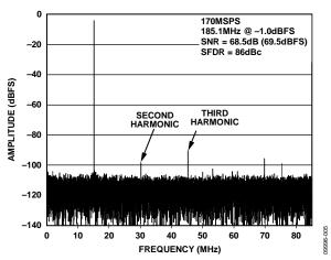
Figure 5. AD9634-170 Single-Tone FFT with  $f_{IN} = 185.1$  MHz
