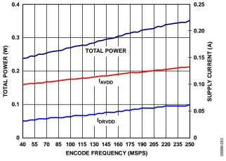
Figure 57. AD9634-250 Power and Current vs. Sample Rate
