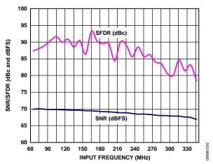
Figure 33. AD9634-250 Single-Tone SNR/SFDR vs. Input Frequency ( $f_{\mathbb{N}}$ ),  $f_{S} = 250$  MSPS
