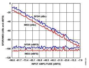
Figure 22. AD9634-210 Two-Tone SFDR/IMD3 vs. Input Amplitude (A<sub>IN</sub>) with  $f_{\rm IN1}=89.12$  MHz,  $f_{\rm IN2}=92.12$  MHz,  $f_{\rm S}=210$  MSPS
