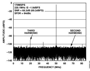
Figure 6. AD9634-170 Single-Tone FFT with  $f_{IN}$  = 220.1 MHz
