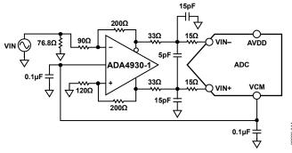
Figure 47. Differential Input Configuration Using the ADA4930-1
