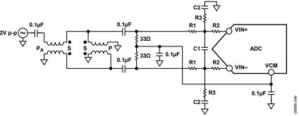
Figure 49. Differential Double Balun Input Configuration
