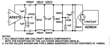
Figure 50. Differential Input Configuration Using the AD8375
