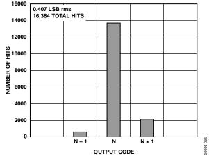
Figure 39. AD9634-250 Grounded Input Histogram,  $f_S = 250$  MSPS
