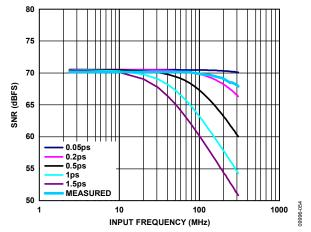
Figure 56. AD9634-250 SNR vs. Input Frequency and Jitter
