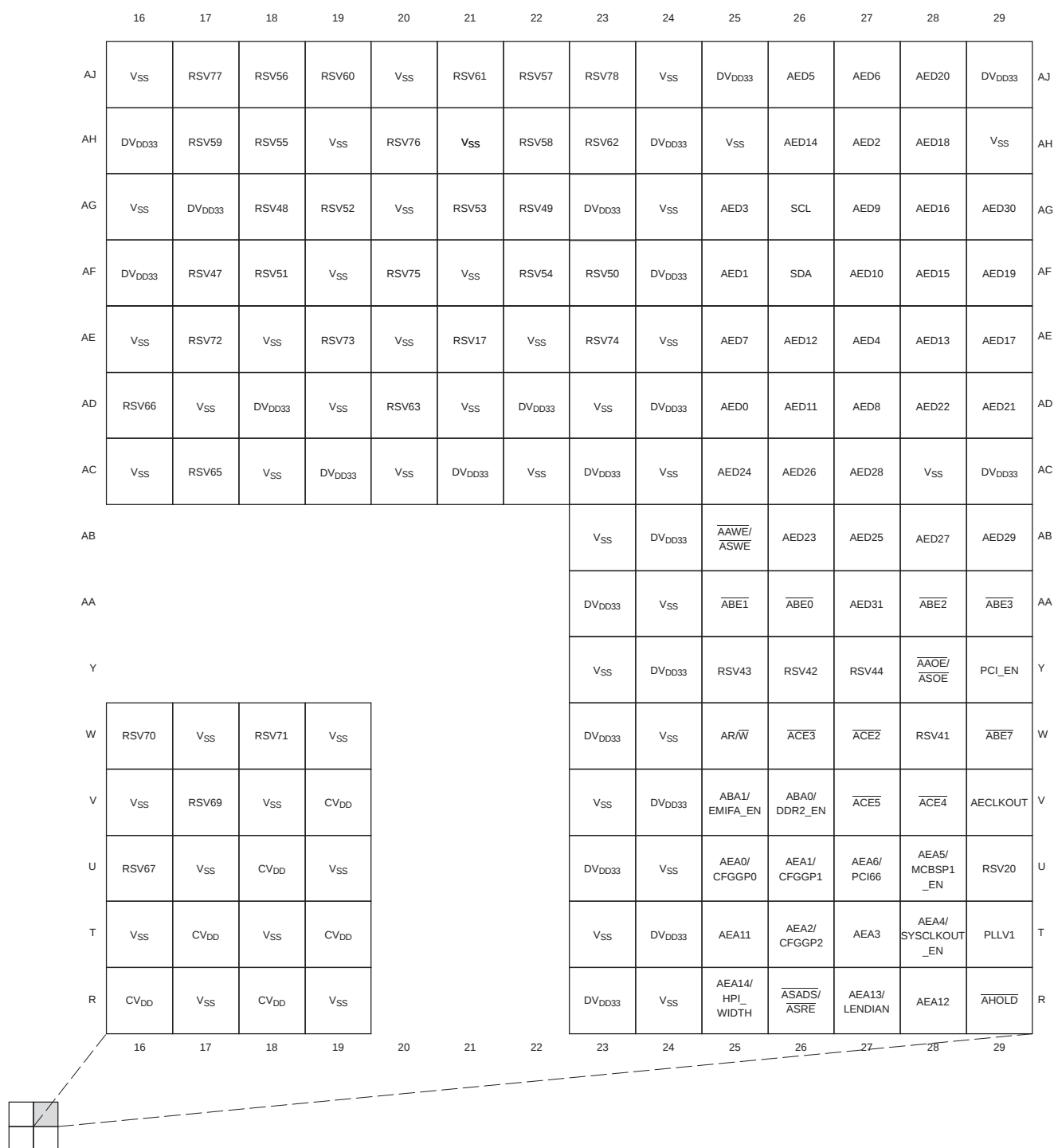
Figure 2-3. C6454 Pin Map (Bottom View) [Quadrant B]
