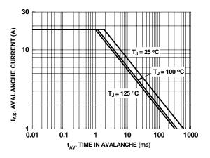
Figure 9. Unclamped Inductive Switching Capability
