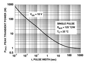
Figure 12. Single Pulse Maximum Power Dissipation
