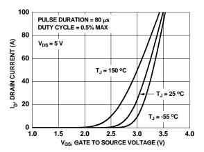
Figure 5. Transfer Characteristics
