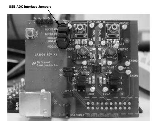
Figure 8. USB Interface ADC Jumpers
