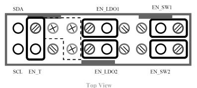
Figure 10. Header Connector
