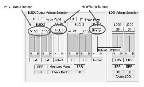
Figure 7. Regulator Output Voltage Selection Interface
