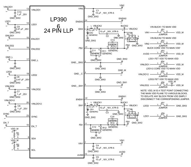
Figure 12. LP3906 Evaluation Board Schematic
