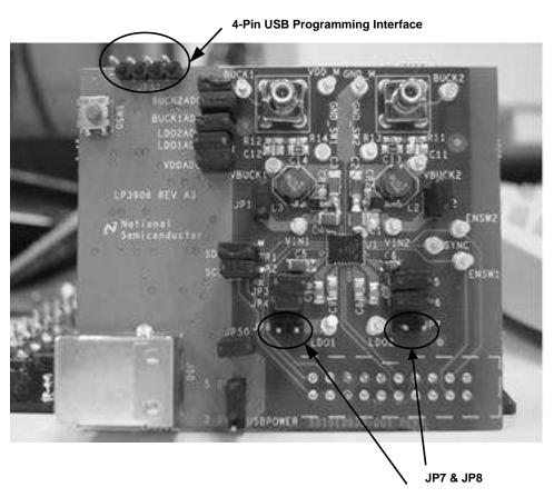
Figure 3. Starting Jumper Settings
