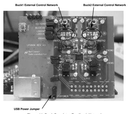
Figure 11. Buck Regulator Feedback Network
