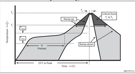
Figure 2. Soldering profile
