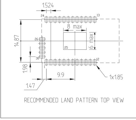
Figure 7. Wi-Fi module footprint
