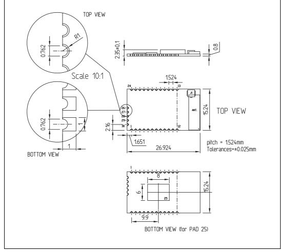
Figure 6. Wi-Fi module dimensions
