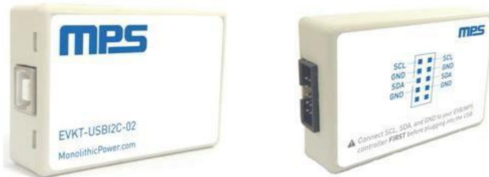
Figure 3: EVKT-USBI2C-02 Communication Interface
