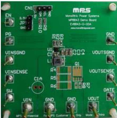
Figure 2: EV8843-G-00A Evaluation Board
