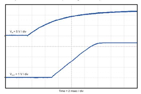
Figure 9. TPS54623EVM-012 Start-Up Relative to  $V_{\text{IN}}$
