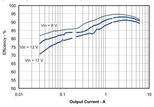
Figure 2. TPS54623EVM-012 Low-Current Efficiency
