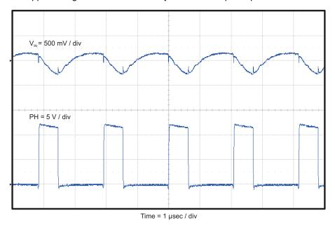
Figure 8. TPS54623EVM-012 Input Ripple
