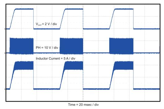
Figure 12. TPS54623EVM-012 Hiccup Mode Current Limit
