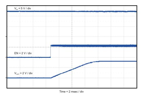
Figure 10. TPS54623EVM-012 Start-Up Relative to Enable
