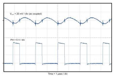
Figure 7. TPS54623EVM-012 Output Ripple
