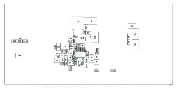
Figure 14. UCC29910AEVM-730 Bottom Assembly Drawing (bottom view)
