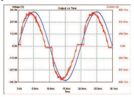
Figure 11. Input Waveforms ( $V_{IN}$  = 230  $V_{AC}$  at 50 Hz,  $I_{O}$  = 1.2 A Test Points: TP1 and TP2)
