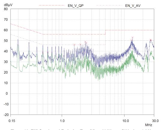
Figure 12. EMI Conducted Emission Test (Vin = 230Vac at 50Hz, Io = 1.2A)
