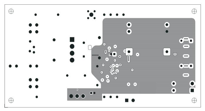
Figure 17. UCC29910AEVM-730 Internal Layer 2 (top view)
