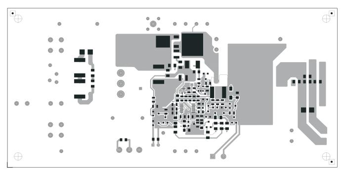
Figure 18. UCC29910AEVM-730 Bottom Copper (top view)
