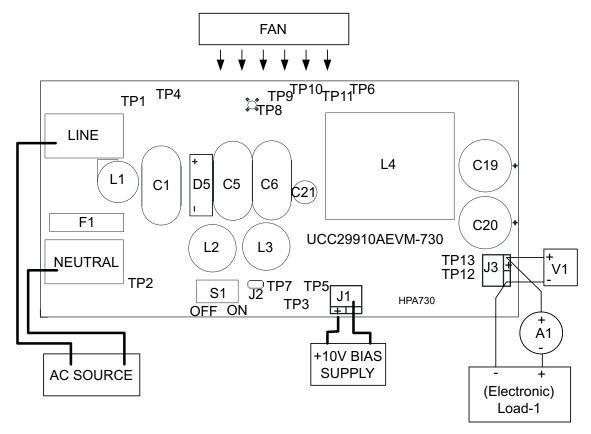
Figure 2. UCC29910AEVM-730 Recommended Test Set Up
