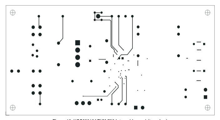
Figure 16. UCC29910AEVM-730 Internal Layer 1 (top view)
