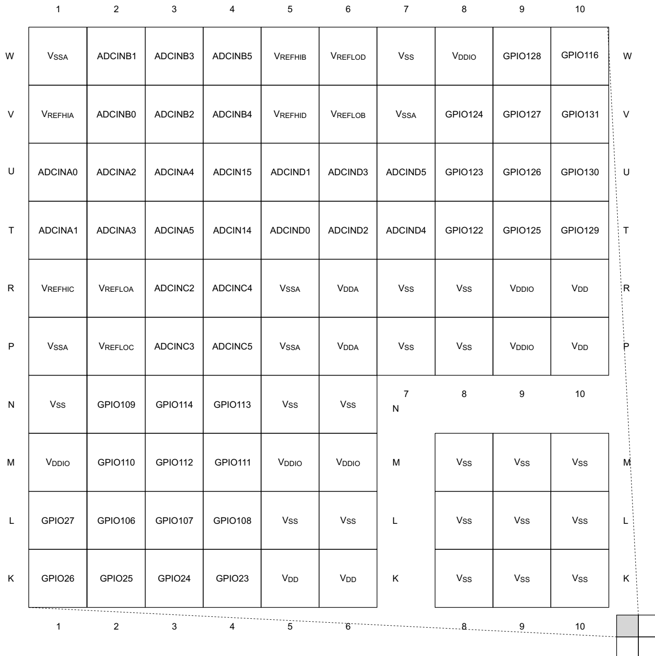
Figure 3-1. 337-Ball ZWT New Fine Pitch Ball Grid Array (Bottom View) – [Quadrant A]
