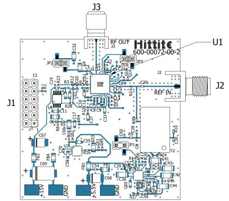
The circuit board used in the application should use RF circuit design techniques. Signal lines should have 50 Ohm impedance while the package ground leads and exposed paddle should be connected directly to the ground plane similar to that shown. A sufficient number of via holes should be used to connect the top and bottom ground planes. The evaluation circuit board shown is available from Hittite upon request.
