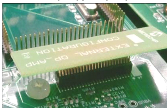
FIGURE 2: EXTERNAL OP AMP CONFIGURATION BOARD
