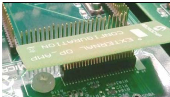
FIGURE 2: EXTERNAL OP AMP CONFIGURATION BOARD
