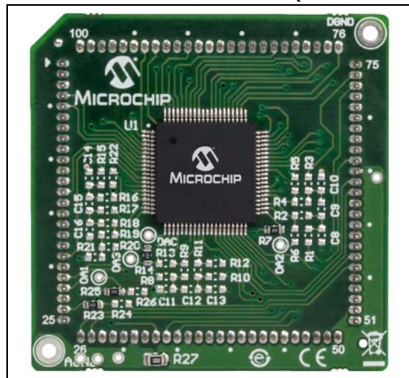
FIGURE 2: EXTERNAL OP AMP CONFIGURATION BOARD
