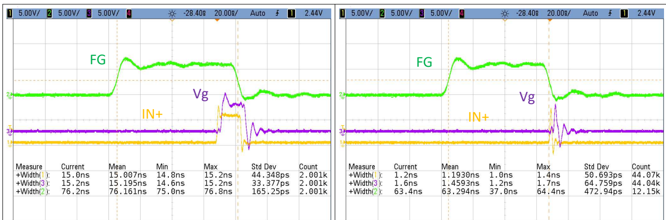
Figure 10. 76 ns Pulse from Function Generator Yielding 15 ns Pulse on the Gate
