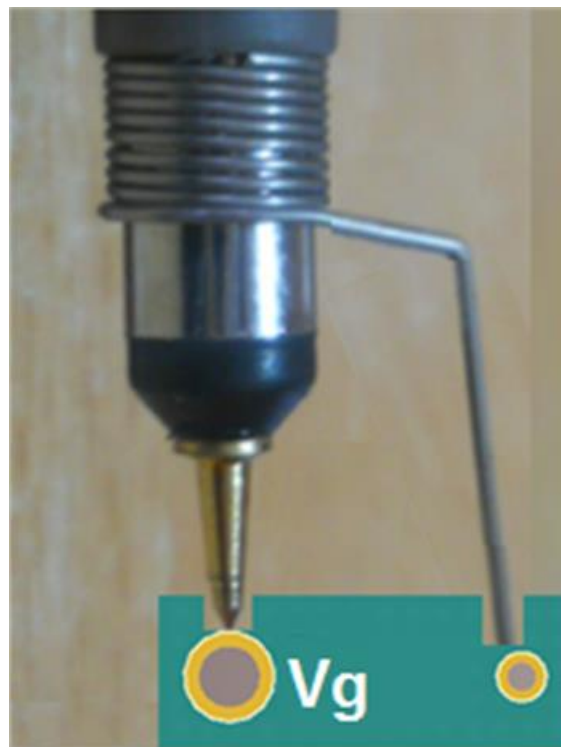
Figure 7. Recommended Use for Ground Spring Clip Test Points
